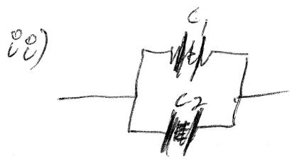
$$C = C_1 + C_2 \quad Z = \frac{-j}{\omega C} = \frac{-j}{\omega(C_1 + C_2)}$$
