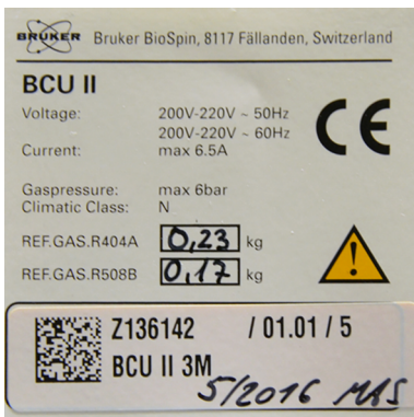
Figure 3.6: BCU II Type 3: 200 – 220 V ~ 50 / 60 Hz, max. 6.5 A
