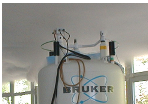
Figure 6.1: Magnet system during a quench
