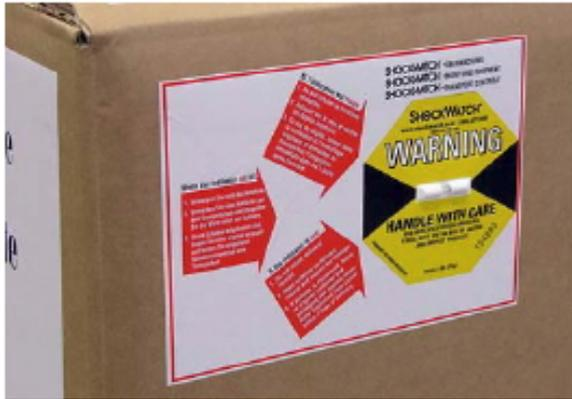
Figure 4.13: Attaching Shockwatch® indicators
