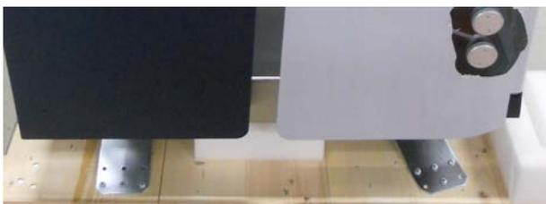
Figure 4.7: Fixing unit on pallet (left side).
