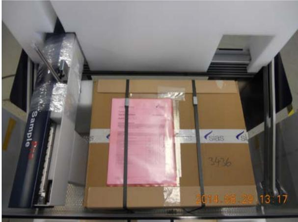
Figure 4.11: Place and fix the accessory box on the deck
