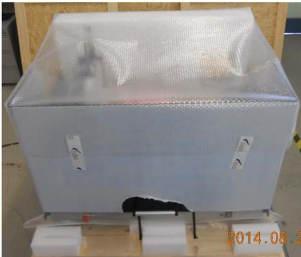
Figure 4.12: Cover the device with bubble foil.
