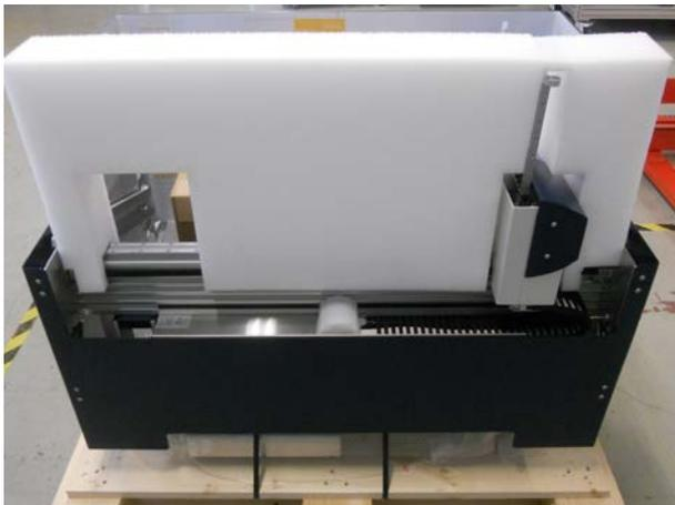
Figure 4.6: Stabilizing the arms and the X-rail with a foam block
