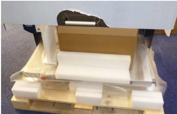
Figure 4.10: Protect front shield with a spacer foam
