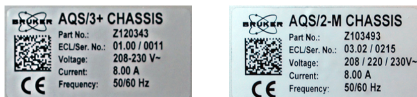
Figure 4.1 AQS/3+ and AQS/2-M chassis rating plate
