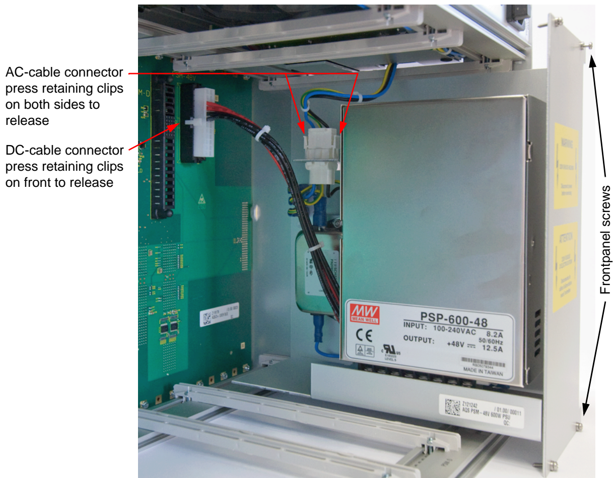
Figure 7.11 PSM-48V removal from mainframe
