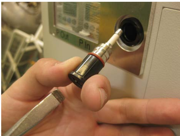
Figure 11.2: Cryocooler Controller Fuse
