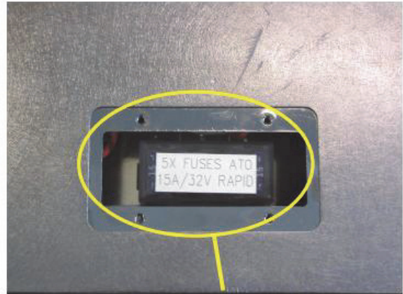
Fuse Box Cover
