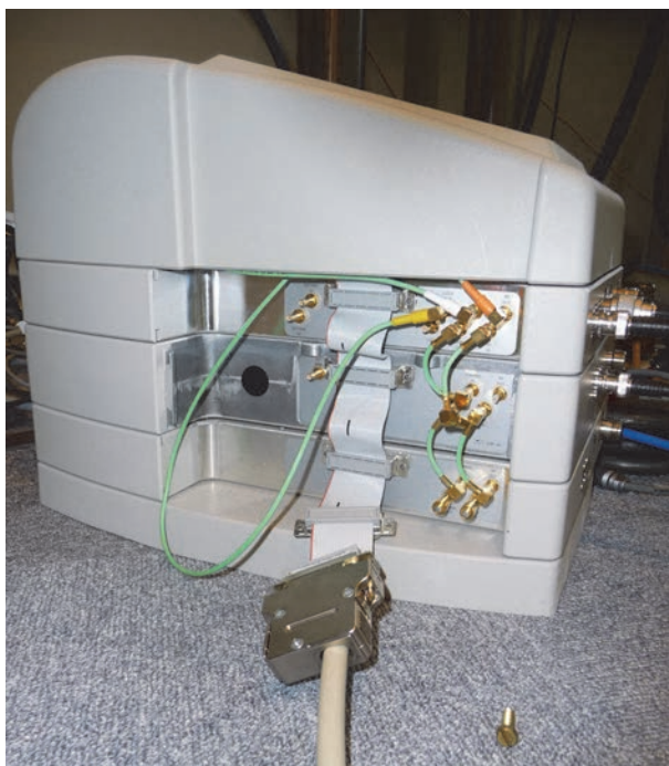
Figure 5.19: Connection of the Combiner to the Preamplifier Flat Band Cable
