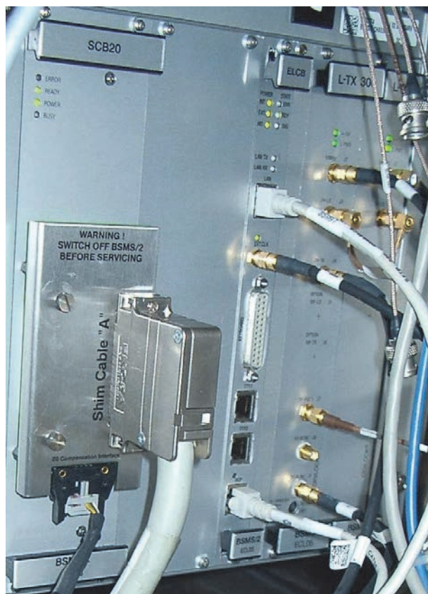
Figure 4.10: BSMS-2 to B0-2 Adaptor Board, Mounted on the Most Right SCB20 Module
