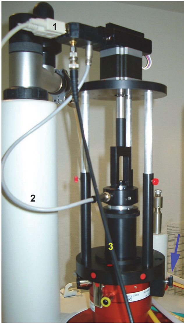
Figure 20.12: Rheo Drive Hardware, Fixed with 2 Screws (blue arrow) on Top of a Magnet
