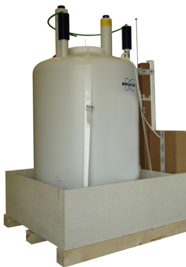
Figure 3.1: Packaging (without surrounding panels)
