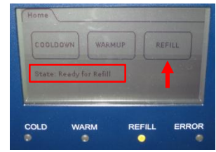
Figure 1. Press <Refill> on the Prodigy unit and wait until the message on the display changes from «Prepare Refill» to «Ready to Refill».
