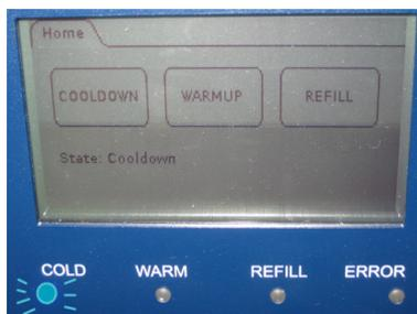
Figure 7.4: Prodigy Unit display: Cooldown state
