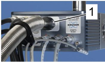
[2] Insert the Transferline (1) to the CryoCoupler on the CryoProbe. Hold the Transferline with one hand and fasten the nut with the other hand.
