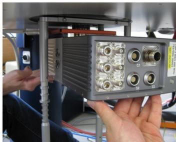
Figure 6.2: Inserting the CryoProbe into the shim system.
