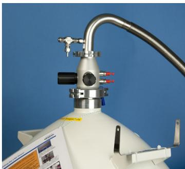
Figure 3.13: Holding clip of the display unit attached to one handle on the LN2 Dewar.
