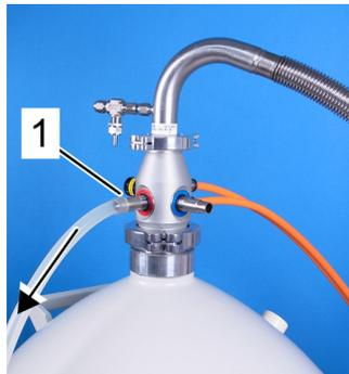
Figure 4.6 LN2 Dewar: Connected white silicone overflow hose.
