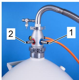
Figure 4.5 LN2 Dewar: LIQUID NITROGEN IN port (blue) (1) and NITROGEN GAS OUT port (red) (2)
