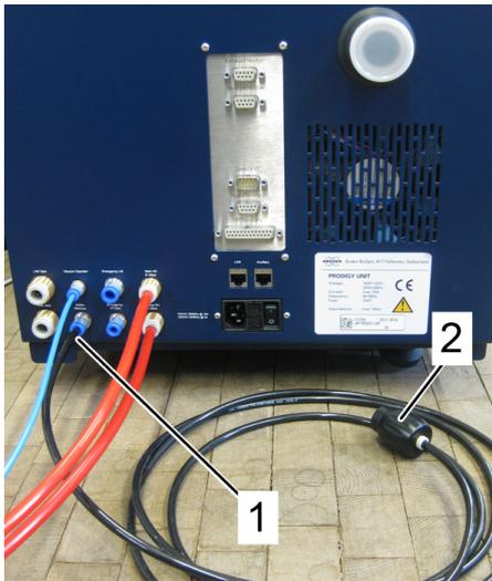
Figure 5.9 Active warmup plug connection.
