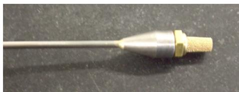
Figure 3.7 Extension piece with filter.
