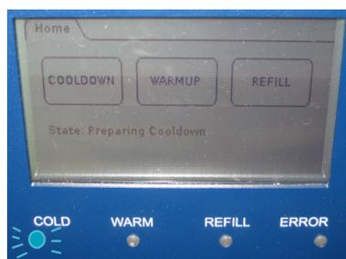
Figure 7.3: Prodigy Unit display: Preparing cooldown
