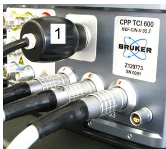
Figure 7.10: Connecting the warmup plug (1)
