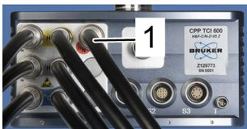
Figure 6.32: Connecting the RF-BNC cables.
