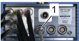
Figure 6.33: Connecting the C1 cable.
