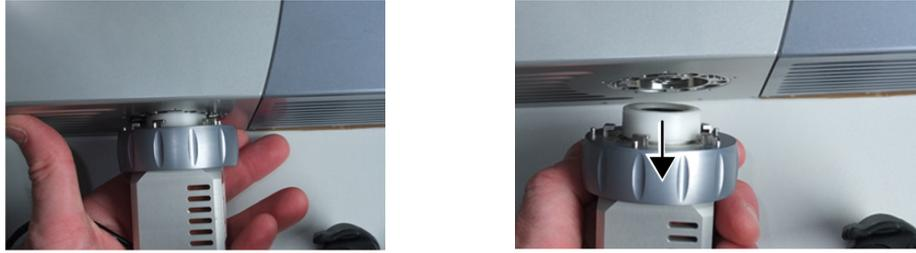
Figure 6.19: Mounting ring can be released. Pulling out the Exhaust Heater/vacuum Operator.
