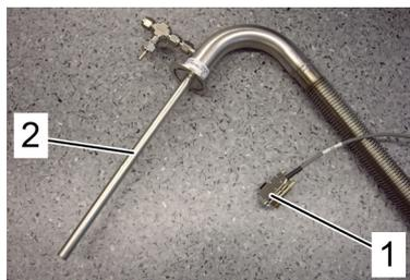
Figure 3.6 Transferline: dewar end connector and Transferline ID cable.
