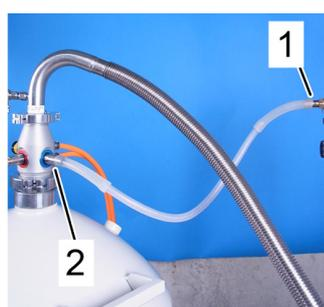
Figure 4.10 LN2 Dewar: Connect the transfer hose to the LIQUID NITROGEN IN port of the LN2 Dewar.
