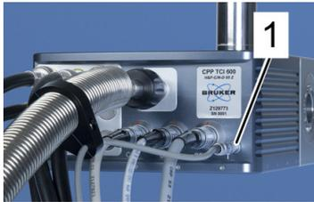
[3] Connect the Transferline ID cable (1) to the front of the CryoProbe.
