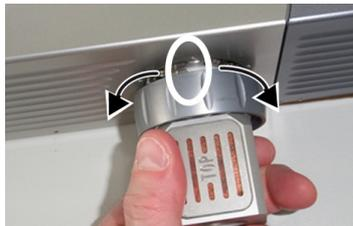
Figure 6.8: Aligning the hooks (2) with the notches (5) of the bayonet plate (4) by turning the mounting ring (1) of the Exhaust Heater.
