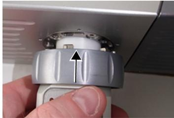
Figure 6.7: Insert and push in the Exhaust Heater.
