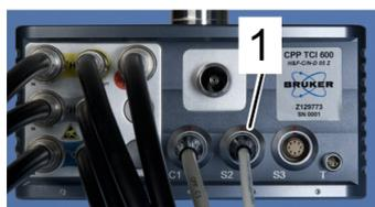
Figure 6.34: Connect the S2 cable.
