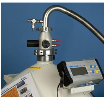
Figure 3.14: Holding clip of the display unit attached to one handle on the LN2 Dewar.
