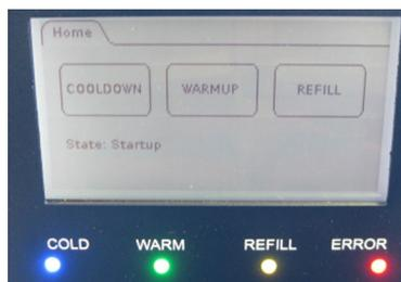
Figure 7.1: Prodigy Unit display and LEDs during startup.
