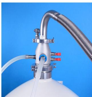
Figure 4.17: LN2 Dewar with connected overflow hose and transfer hose.
