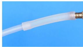
Figure 4.7: Liquid nitrogen extraction port of the Transport dewar (exemplary illustration) with attached silicone hose and PTFE transfer hose
