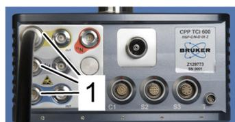
Figure 6.30: Connecting the RFN cables.
