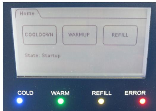
Figure 5.2: Prodigy Unit touch screen interface and LED display.
