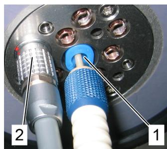
Figure 6.24: Bottom of CryoProbe with VT adaptor and sample heater cable.
