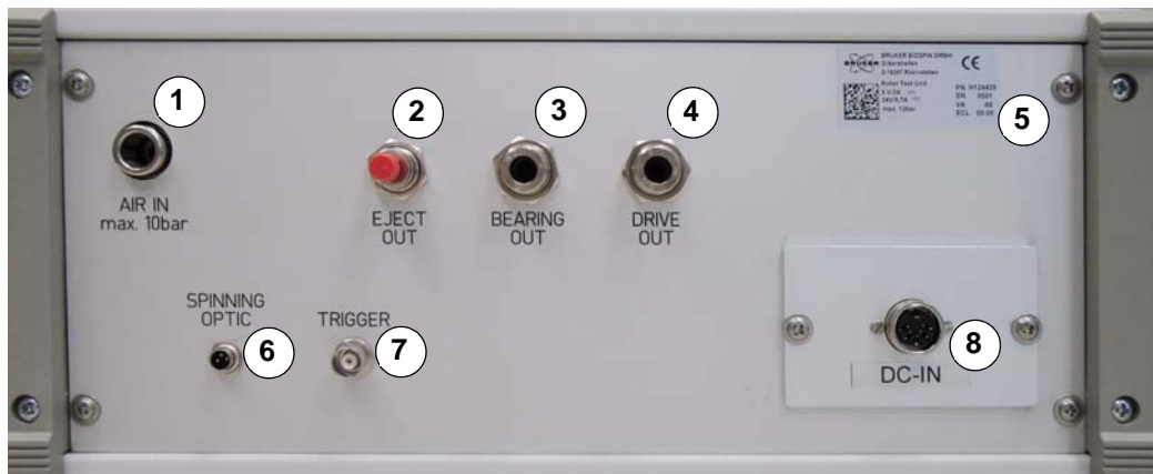
Figure 5.2 Rotor Test Station - Rear Side
