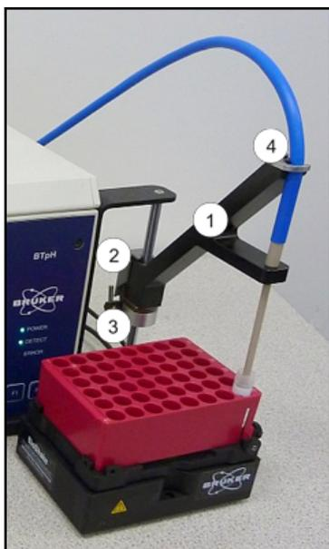
Figure 5.5: The pH Sensor Stand
