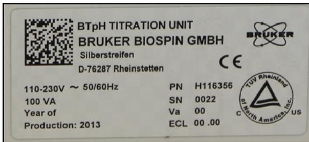
Figure 4.2: BTpH Titration Unit Rating Plate
