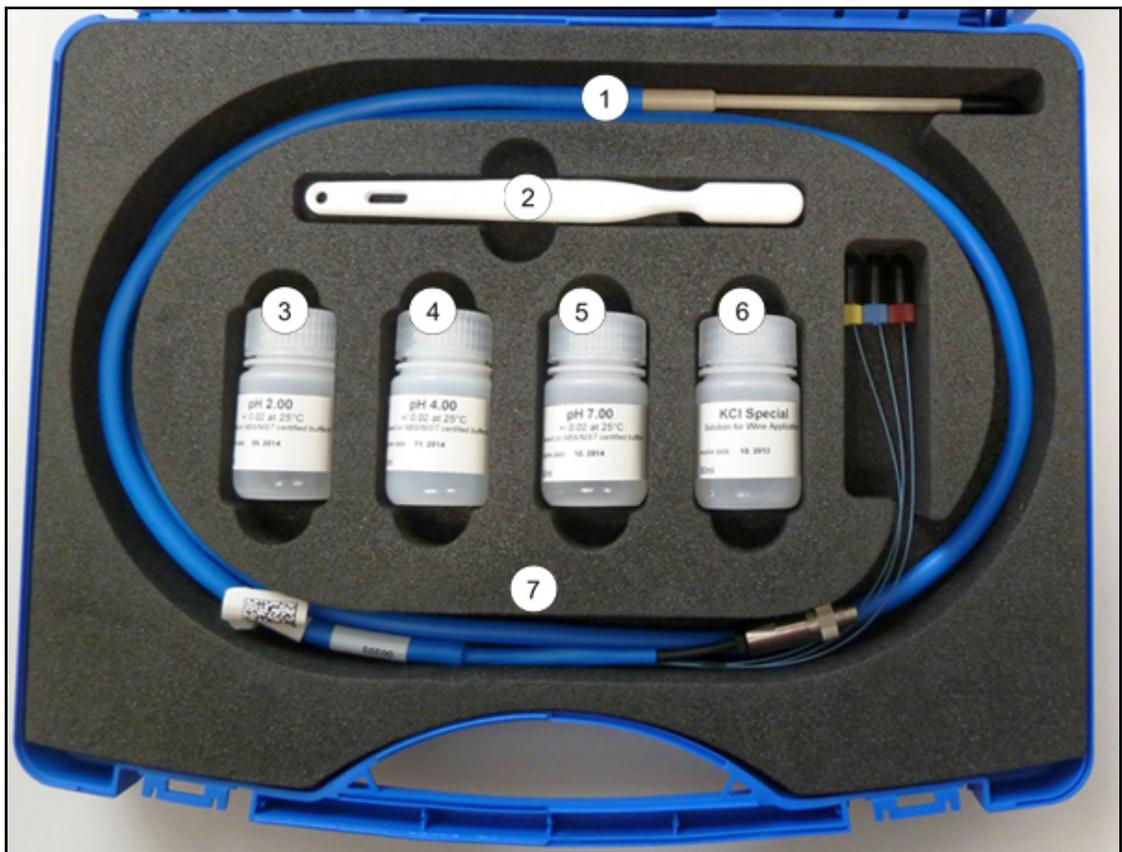
Figure 4.1: The pH Sensor Kit
