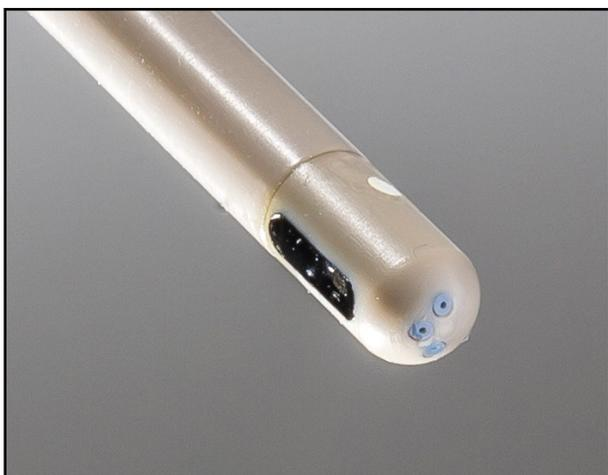
Figure 8.3: The pH Probe Tip
