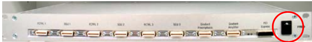
Figure 8.1 Location of the ON/OFF Switch
