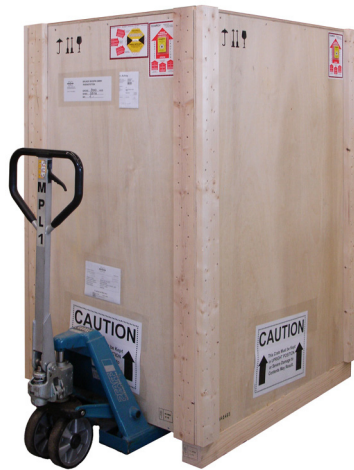
Figure 3.2: Transportation by forklift - front side
