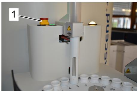
Figure 3.1: Emergency stop button (1) of the SampleCase
