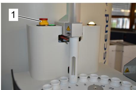
Figure 6.2: Emergency stop button (1) of SampleCase
