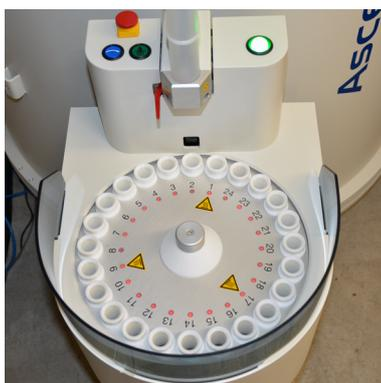
Figure 5.3: SampleCase heated carousel with 24 positions for samples to be individually heated
