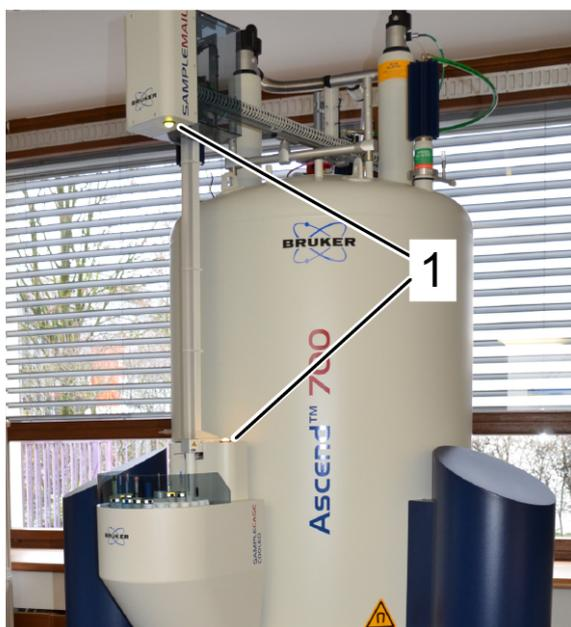
Figure 6.1: LED interface (1) at SampleMail and SampleCase highlights the operating state.
