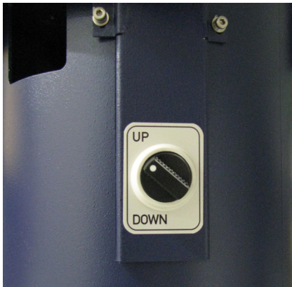
Figure 5.1: Start the Magnet Stand
