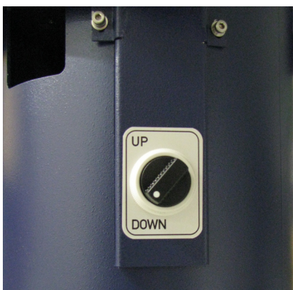
Figure 5.2: Stop the Magnet Stand
