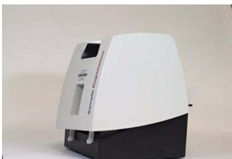
5. Carefully lift the cover out of the base.
