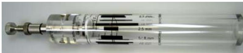
Figure 2.2 Sample Tube Adjustment Device
