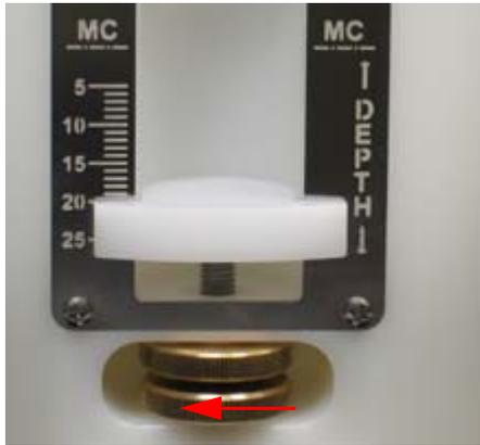
Figure 7.4 Loosening the Knurled Screws
