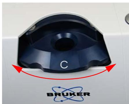
Select the desired position of the rotary disk by rotating it until it locks in place. You will hear an audible click.
