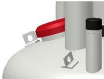
Figure 3.4: Attachment points for lifting equipment
