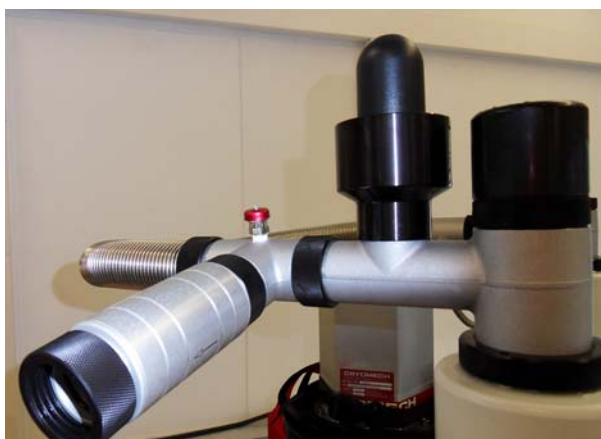
Figure 9.4: DNP sweep valve on the helium flow system
