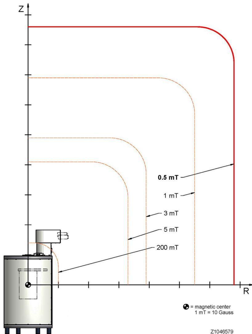
Figure A.3: Fringe field plot of the EPR 12T magnet system
