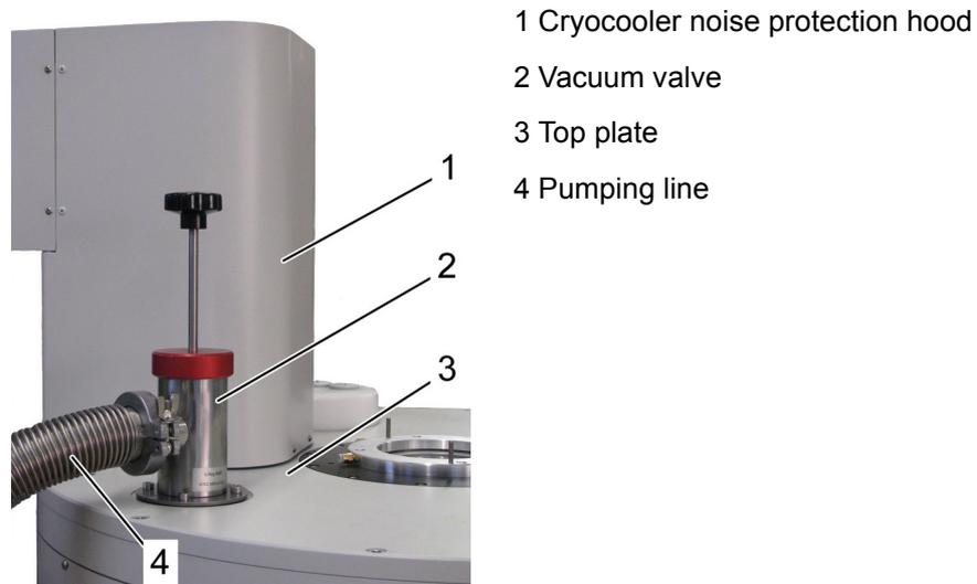
Figure 5.2: Vacuum valve mounted at the magnet system
