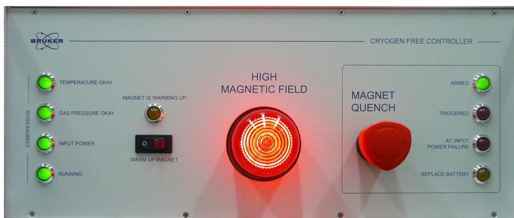
Figure 5.16: Energizing the magnet and checking the indicator
