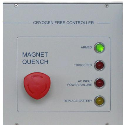
Figure 5.15: Emergency button MAGNET QUENCH on the BCFC front panel
