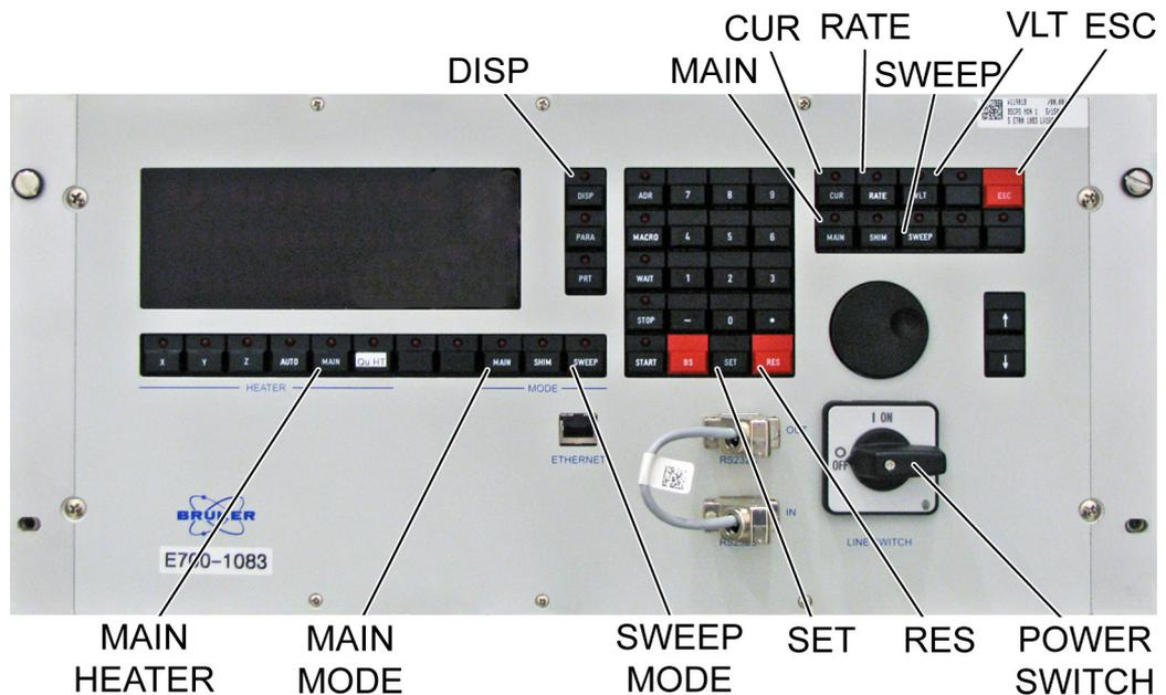
Figure 5.11: Front panel of the power supply E700–1083
