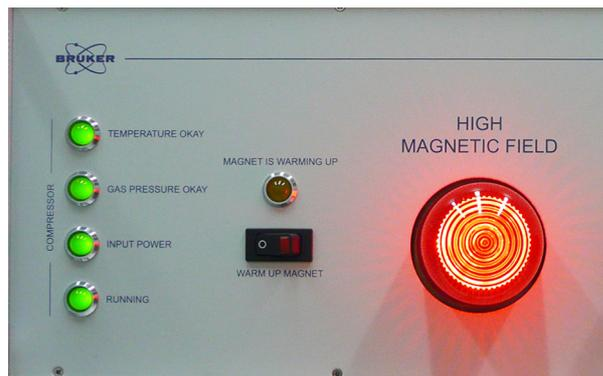
Figure 5.17: Quenching the magnet in an emergency case
