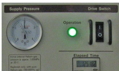
Start the compressor CNA-61 using the "DRIVE SWITCH".
