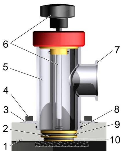
3. Install the valve stem (6) onto the sealing plug (2) and tighten it slightly. Do not yet fix the valve operator body (5) to the cryostat.
