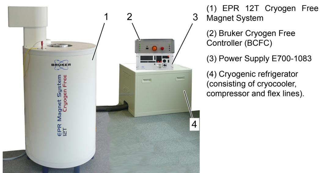
Figure 1.1: Overview of the EPR magnet system
