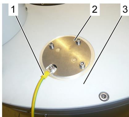
Figure 5.7: Mounting the earthing cable
