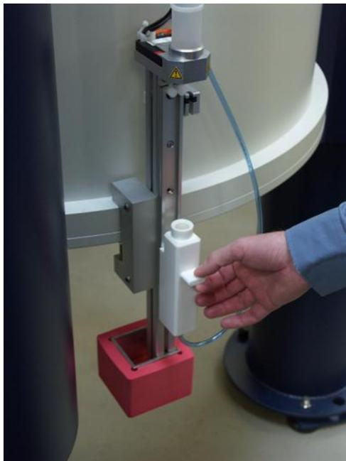
Take hold of the slider and pull it down to the stop.
