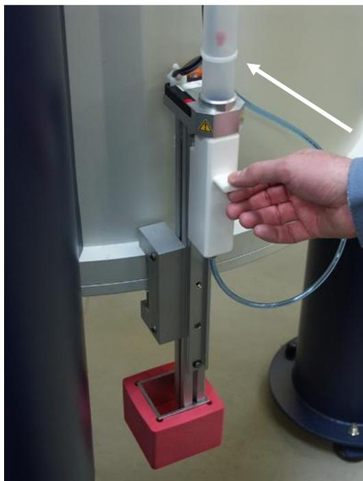
As soon as the sample has arrived in the loading compartment (arrow), open the latter downwards.
