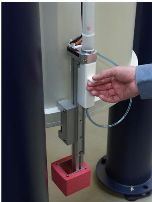
Push the slider right up to the stop, and the transport will now be triggered.
