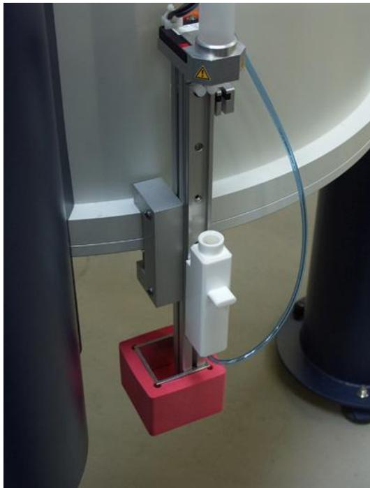
If the compartment is not to be reloaded for a further experiment, it is important that the slider should be left open.
