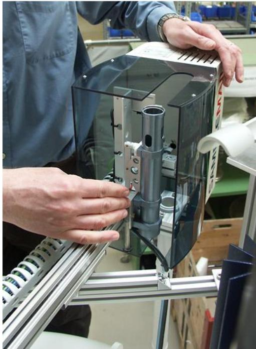
Push the tube completely inwards into the housing
