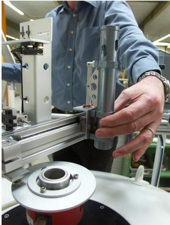
Push the guide tube away from the BST. Always hold the tube close to the linear guide.
