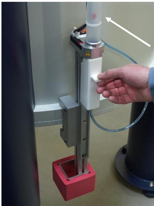
As soon as the sample can be seen to have arrived in the loading compartment (arrow), open the latter downwards.
