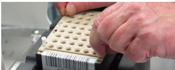
8. Hold the tray by the small white lifting arms and insert the tray into the cooling rack.
