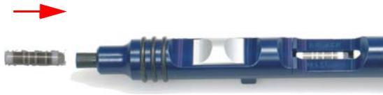
3. Remove the rotor from the slot and insert it, cap first, into the flexible nozzle.
