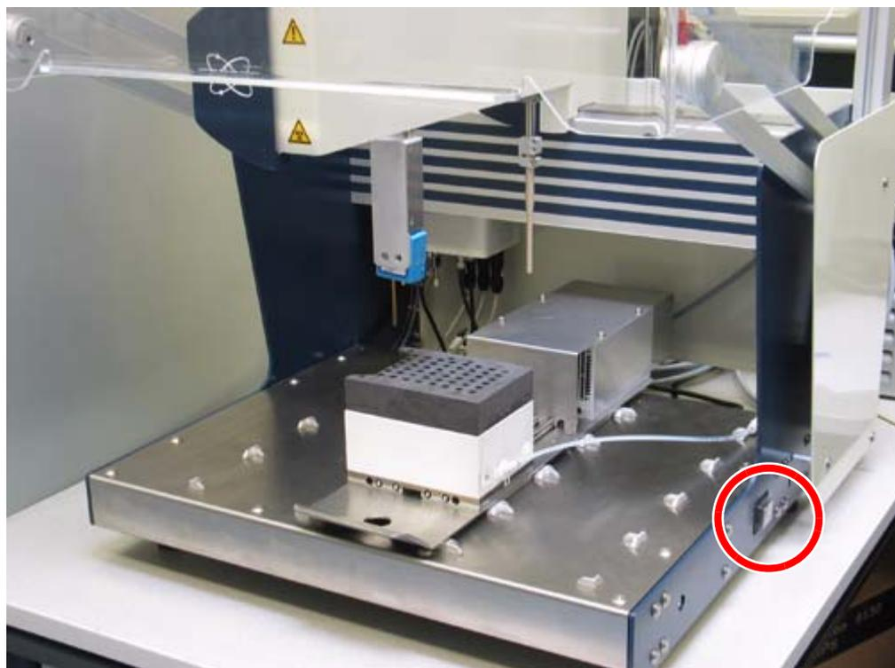
Figure 3.1 The Robot ON/OFF Switch
