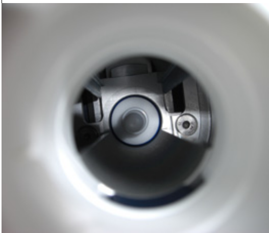
Figure 11.1 Sample Stuck in Magnet
