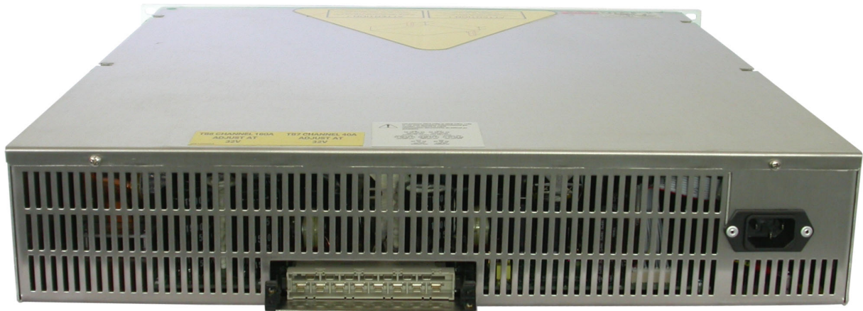
Figure 4.9. Power Supply Rear Panel View
