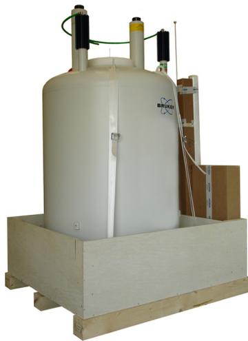
The cryostat is supplied in a wooden box on a pallet. It is secured inside with straps against tilting and moving.
