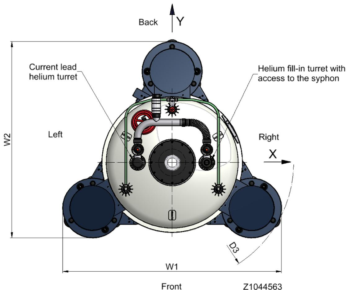
Figure A.2: Dimension Cryostat - Top View
