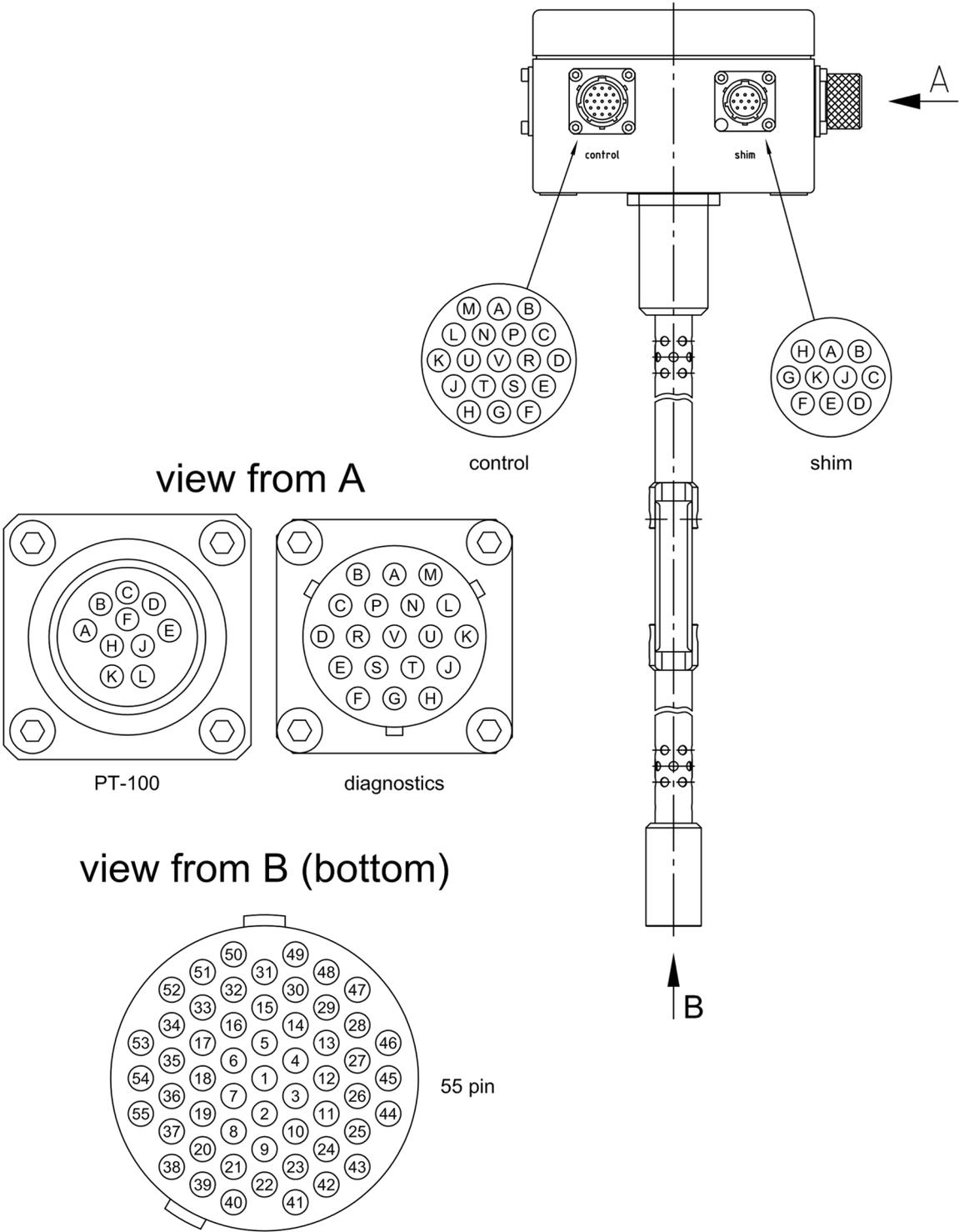
Figure A.8: Current Lead 55 pins
