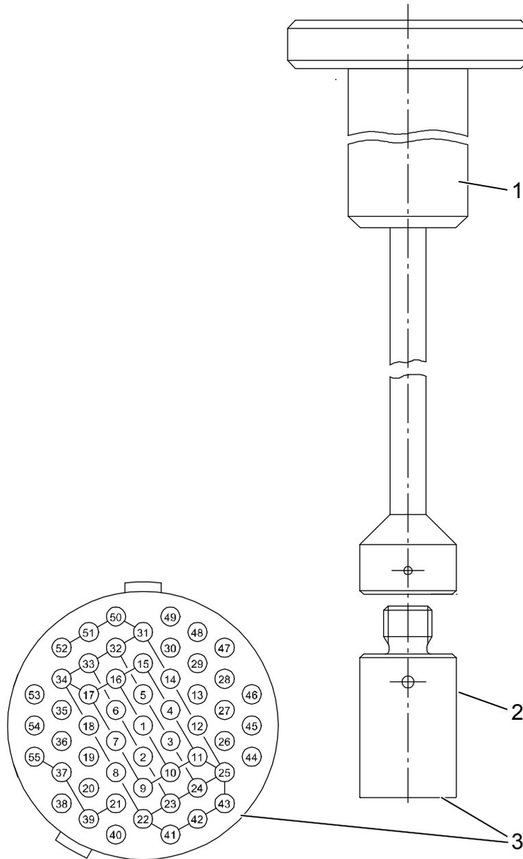
Figure A.12: Shorting Plug 55 pins
