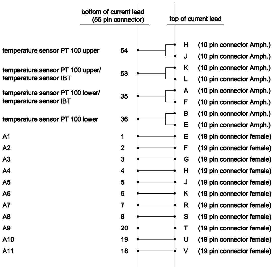
Figure A.11: Wiring Diagram Magnet - Diagnostic and Temperature Sensors
