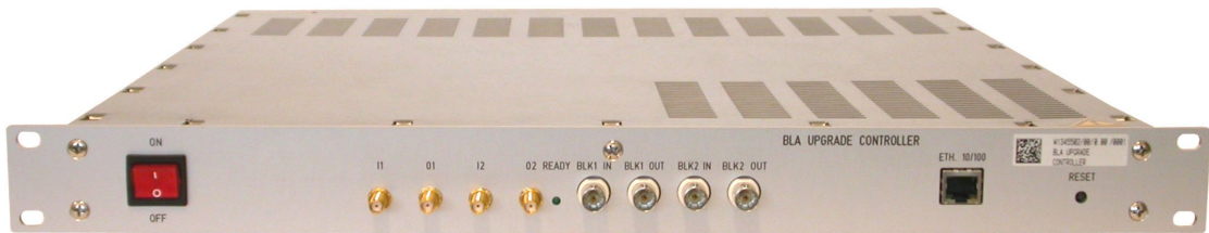
Figure 5.3: BLA Upgrade Controller Front Panel View
