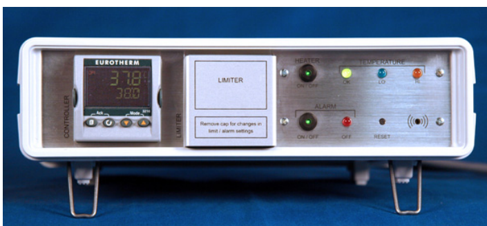
Figure 4.11: On the MRI Temperature Control Unit the left LED display shows the actual temperature at the interface, while the right LED display (normally covered) shows the temperature of a second independent sensor (for safety reasons).
