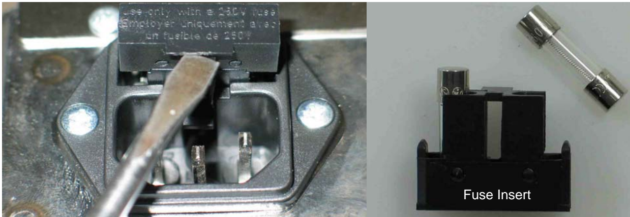
Figure 14.10: Replacing the Control Unit Fuse
