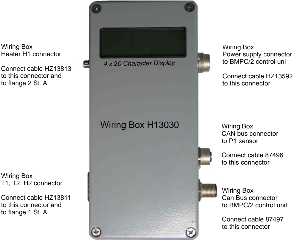
Figure 5.6: BMPC/2 Wiring Box
