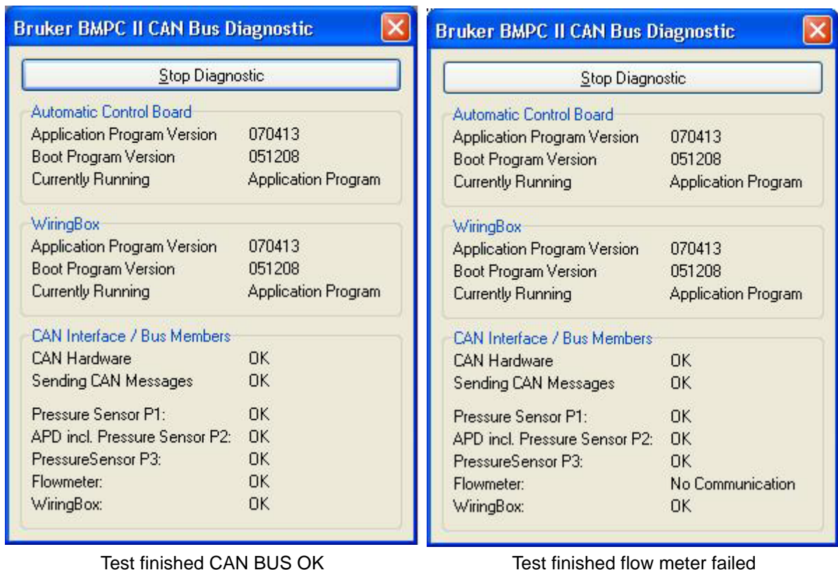
Figure 11.3: Setup Tool - Can Bus Diagnostic
