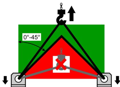
Figure 3.3: Attachment points for lifting equipment
