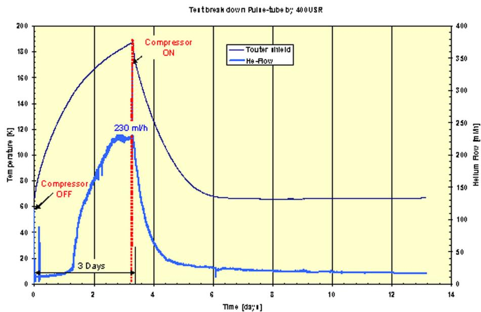
Figure 6.2: Temperature profile during Cryogenic Refrigerator failure
