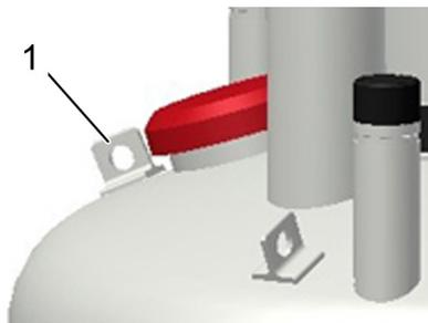
1. Exclusively use the marked eyelets (1) as attachment points for the lifting equipment.
