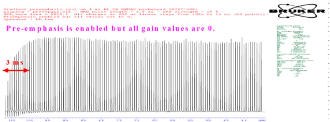
Figure 6.2. The same test recorded with an HR-MAS Z gradient probe but the first step and the first increment are set to 100 \mu s.
