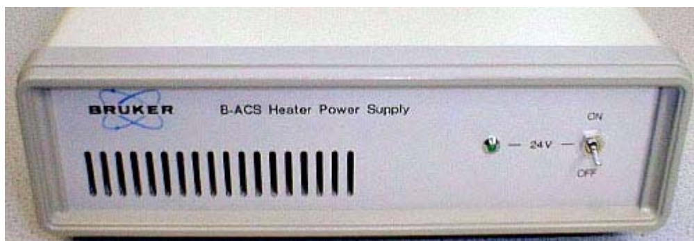
Figure 3.5. Front View of the B-ACS Heater Supply 2
