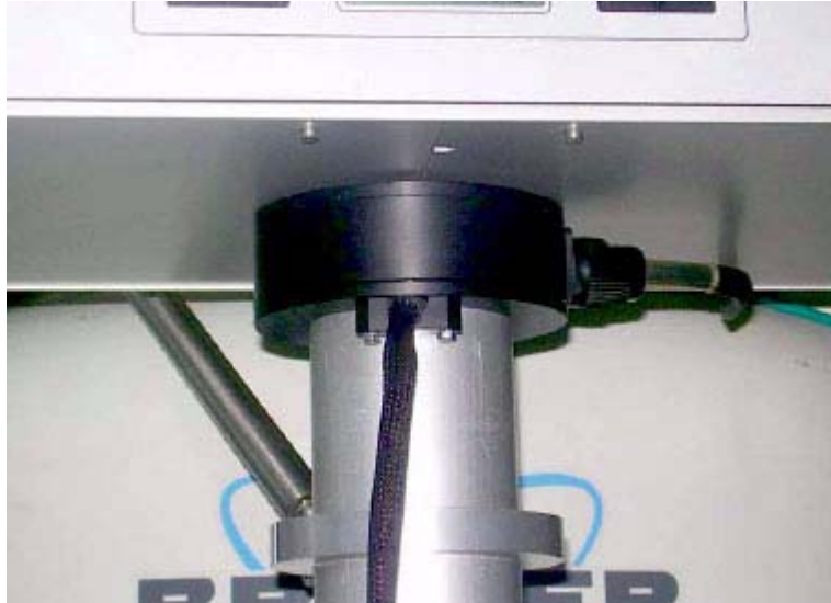
Figure 3.2. Sliding Ring Placement
