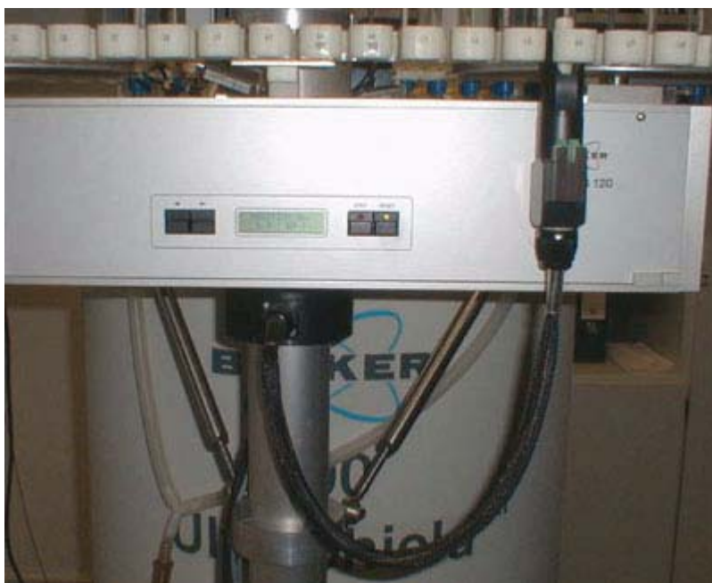
Figure 1.1. B-ACS with Sample Heater
