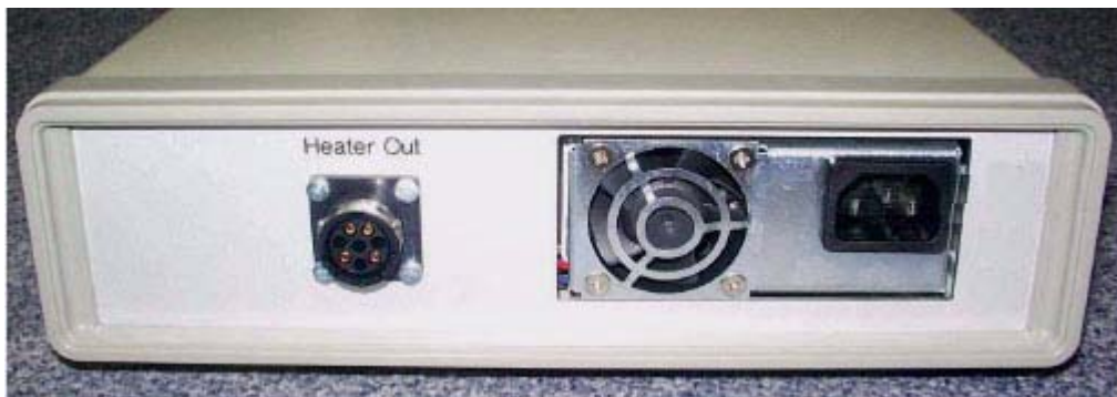
Figure 3.4. Rear View of the B-ACS Heater Supply 2
