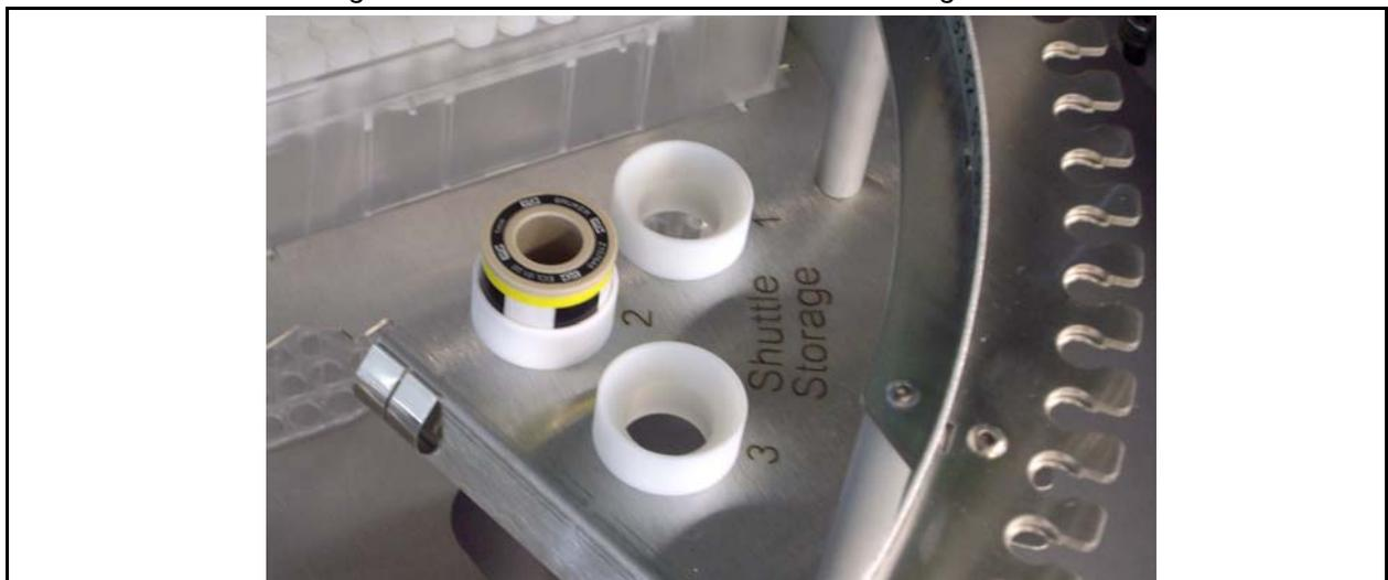
**Correct Placing of the Tubes on the Grate**
