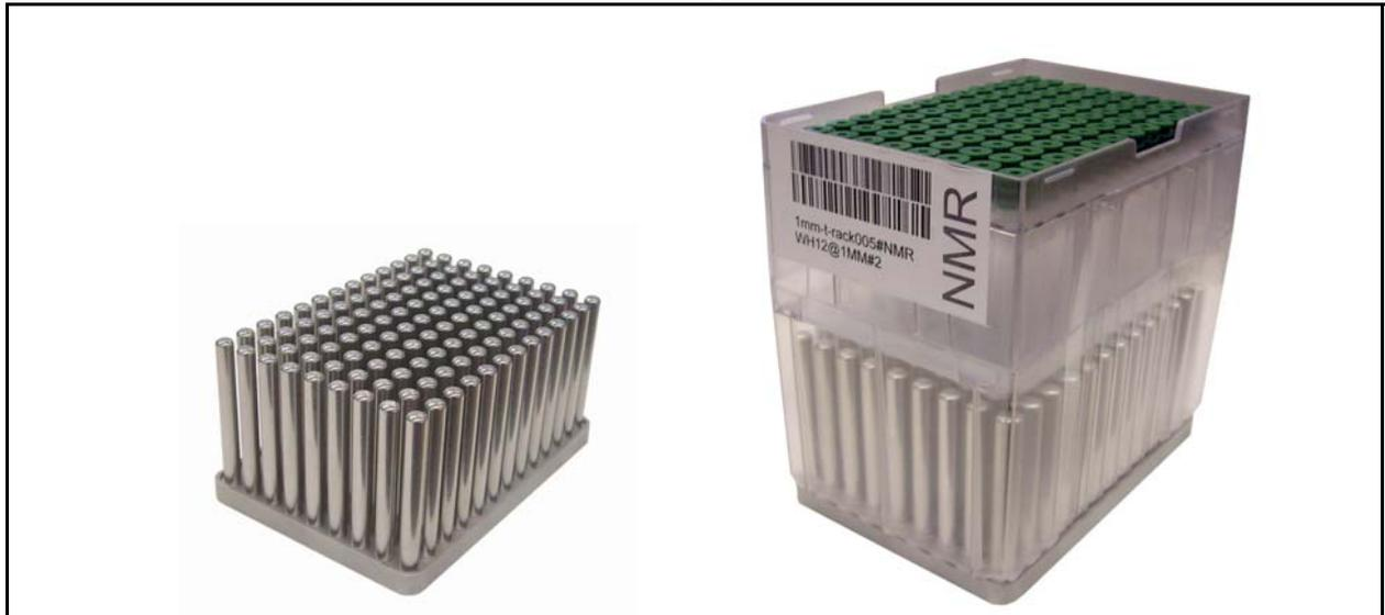
Since the heat exchanger has a much bigger mass than the rack with the tubes, the temperature stays constant when inserting and removing racks. The rack slots do not need to be covered when not in use.
