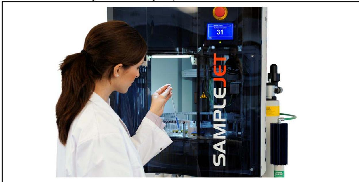
To access a sample in the openshop ring storage use the „Load Sample“ function in the „Main menu“ of the SAMPLEJET display. This will rotate the chosen sample position to the front door.
