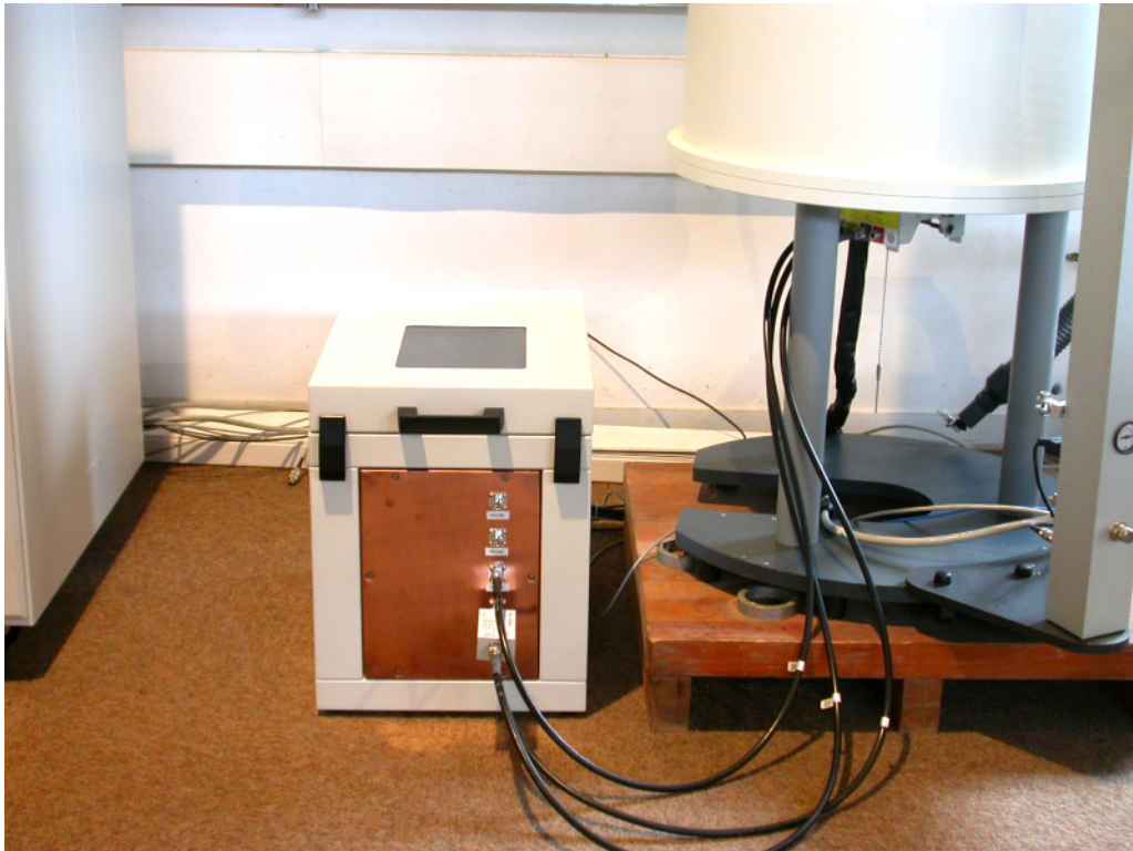
8. The HPPR Faraday cage connected to the magnet is ready to function.
