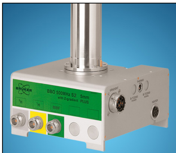
Figure 4.7: Example of a Broadband Probe
