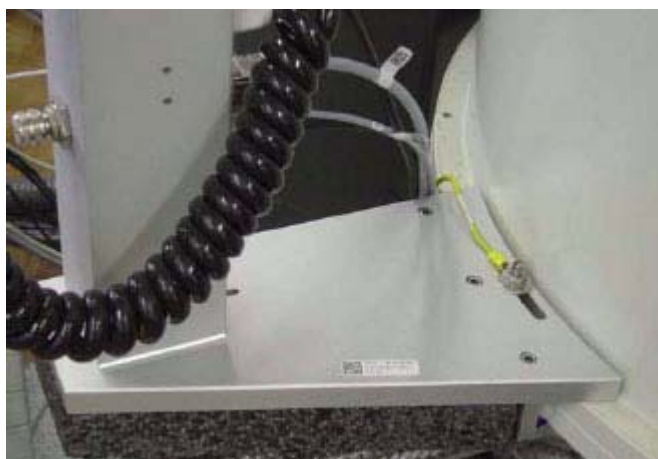
Figure 3.12. Mounting Sample Changer to Magnet with Vibration Dampers
