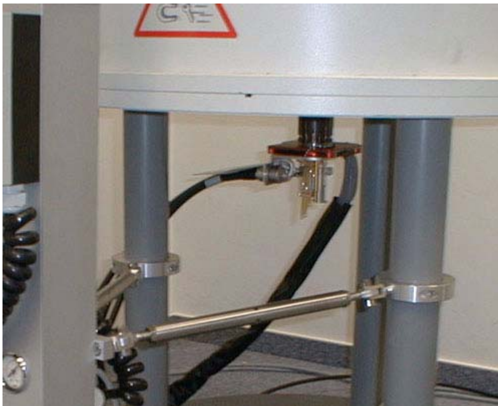
Figure 3.11. Adjustable Arm Assembly for Bottom of B-ACS
