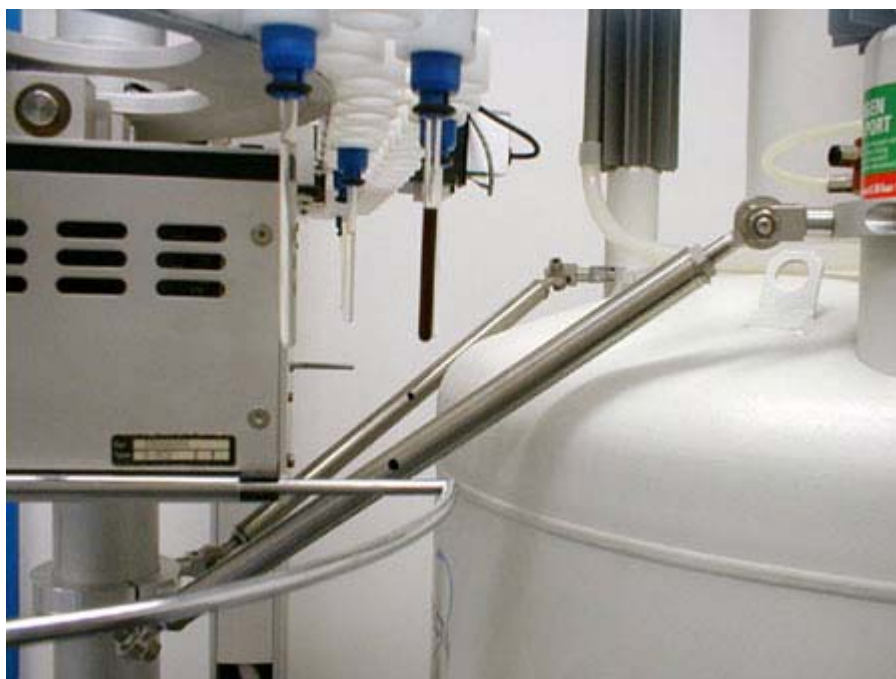
Figure 3.8. Adjustable Arm Assembly for Magnets with N2 Tower
