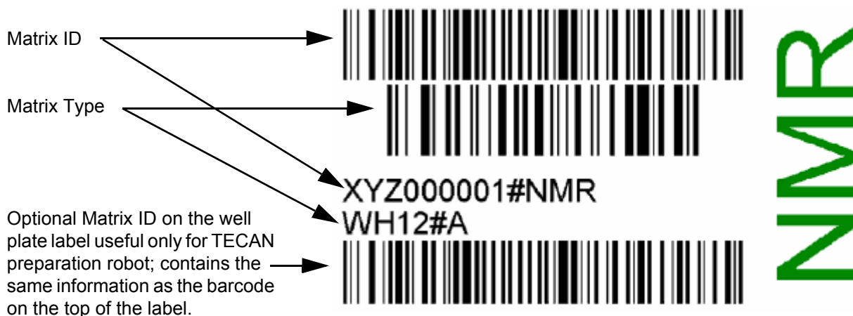
Figure 3.1. Example of the Matrix ID and Matrix Type on a Well Plate Label
