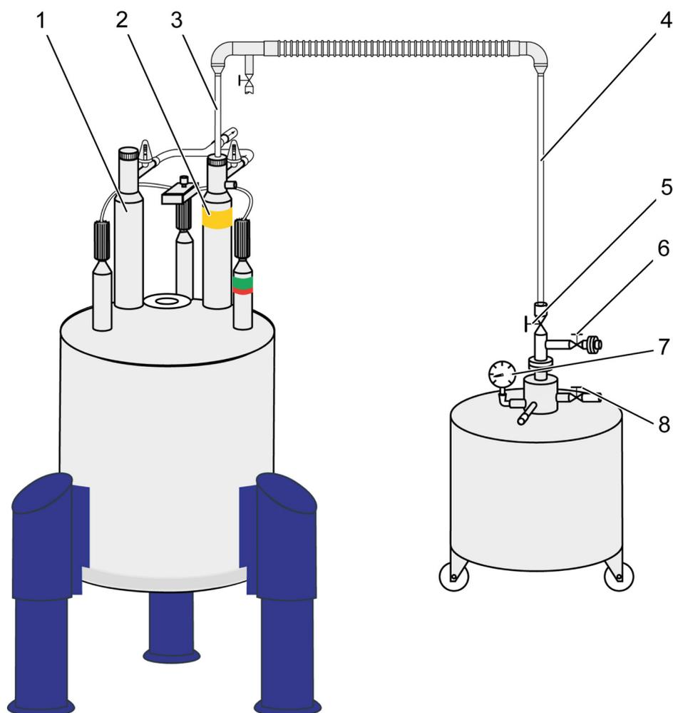
Figure 1.4: Setup of the magnet system during helium refilling procedure
