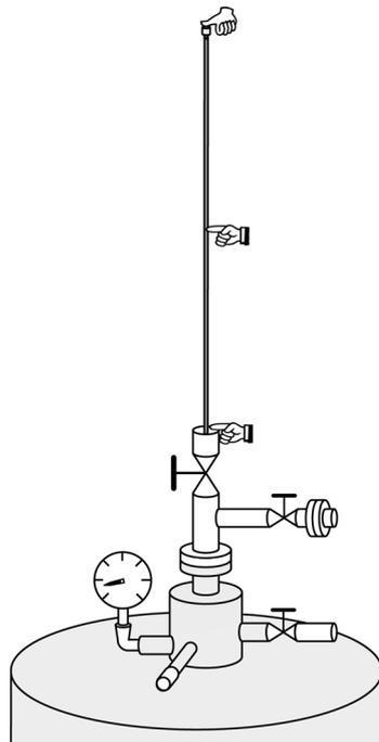
Figure 4.8: Fluid level measurement in the transportation dewar – step 3
