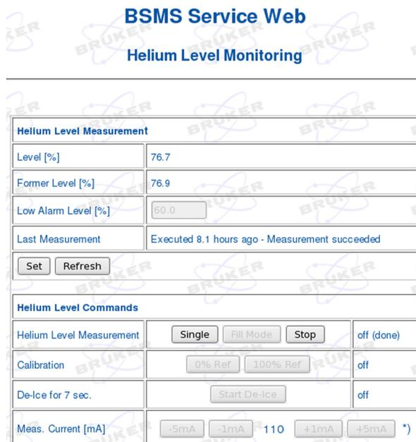
Figure 4.5: User interface of the BSMS Service Web – helium level monitoring
