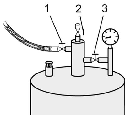
Figure 3.14: Nitrogen refilling procedure – step 7
