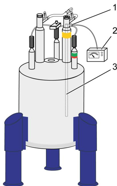
The magnet system provides a built-in Helium Level Sensor (3) to measure the fluid level. It is connected to the BSMS Service Web, where the measured value can be displayed.
