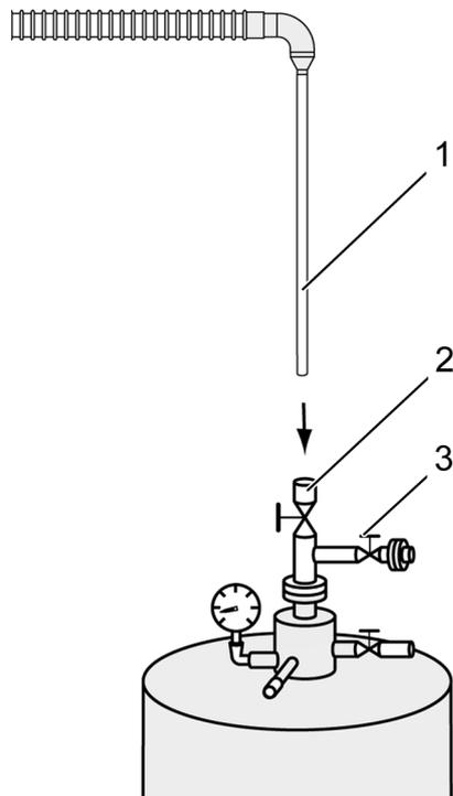
Figure 4.15: Helium refilling procedure – step 6
