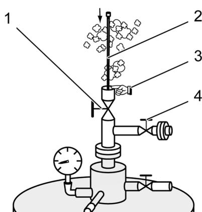
1. Open the pressure regulator valve (4) to release the pressure in the transportation dewar.
