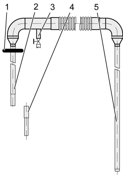
For the transfer of liquid helium a helium transfer line is necessary. The helium transfer line is vacuum-insulated and the vacuum has to be refreshed regularly using a vacuum pump at the vacuum valve (3) of the transfer line.
