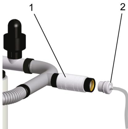
Figure 4.11: Helium refilling procedure – step 2
