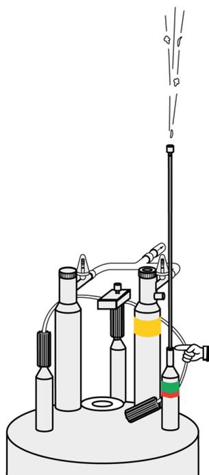
Figure 3.5: Fluid level measurement in the nitrogen vessel – step 1
