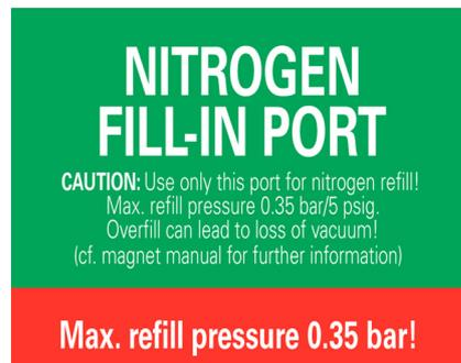
The nitrogen fill-in turret on the magnet system is marked with a green and red colored label.
