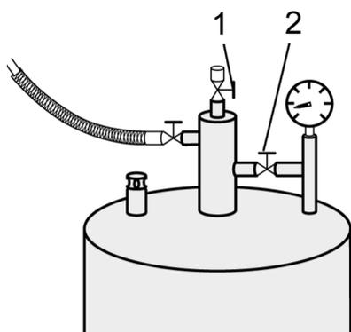
Figure 3.8: Nitrogen refilling procedure – step 1
