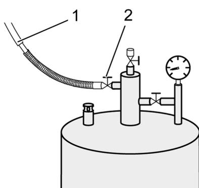
Figure 3.11: Nitrogen refilling procedure – step 4
