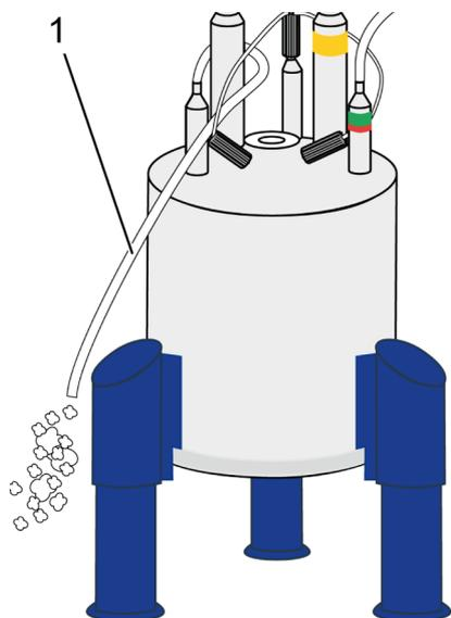
Figure 3.13: Nitrogen refilling procedure – step 6
