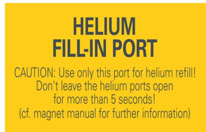
The helium fill-in turret is marked on the magnet system with a yellow label.
