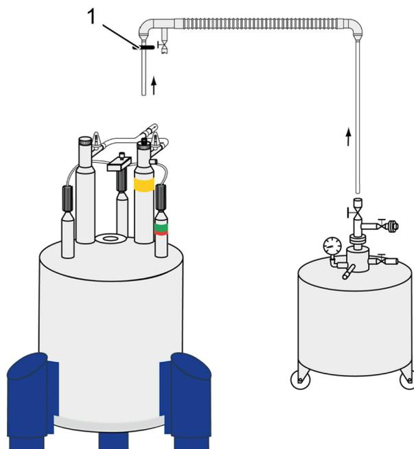
Figure 4.18: Helium refilling procedure – step 9
