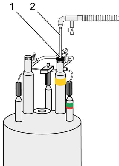
Figure 4.16: Helium refilling procedure – step 7
