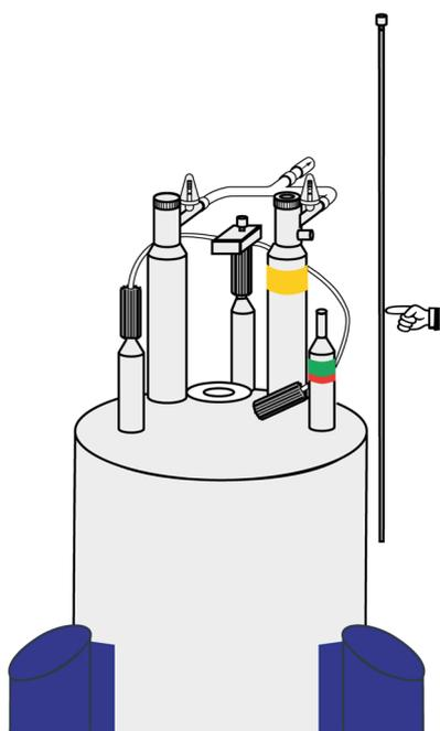
Figure 3.6: Fluid level measurement in the nitrogen vessel – step 2
