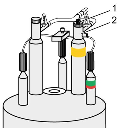
Figure 4.13: Helium refilling procedure – step 4
