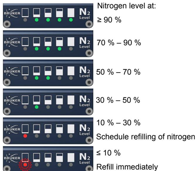
Figure 3.4: Display of the Nitrogen Level Sensor
