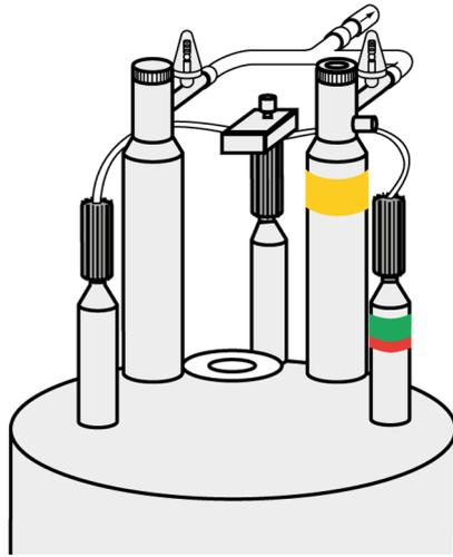
Figure 3.7: Fluid level measurement in the nitrogen vessel – step 3
