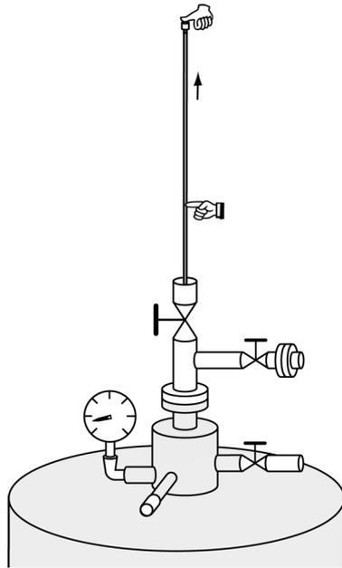
Figure 4.7: Fluid level measurement in the transportation dewar – step 2
