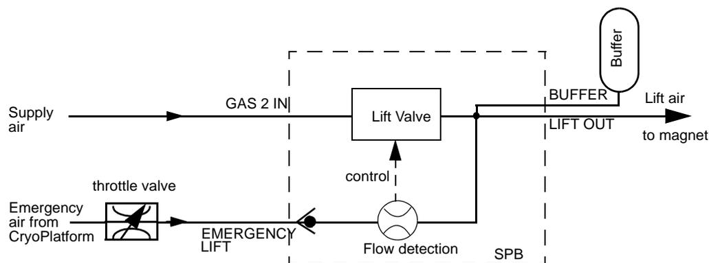
Figure 18.11 Block diagram emergency lift detection
