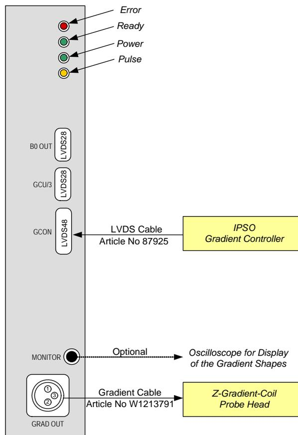
Figure 12.2 GAB/2 in an AVANCE spectrometer with IPSO
