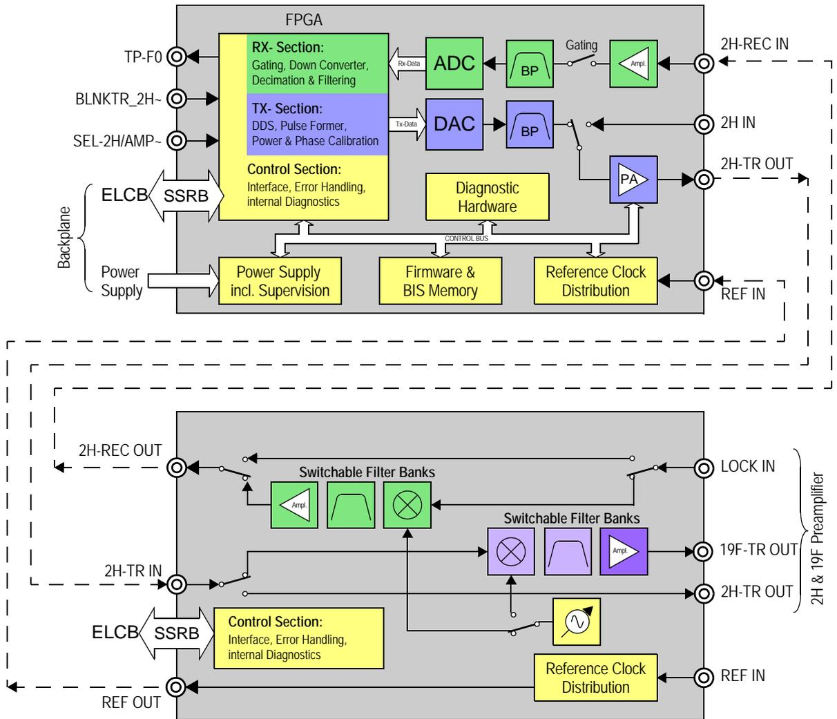
Figure 13.4 Block Diagram with optional L-19F unit
