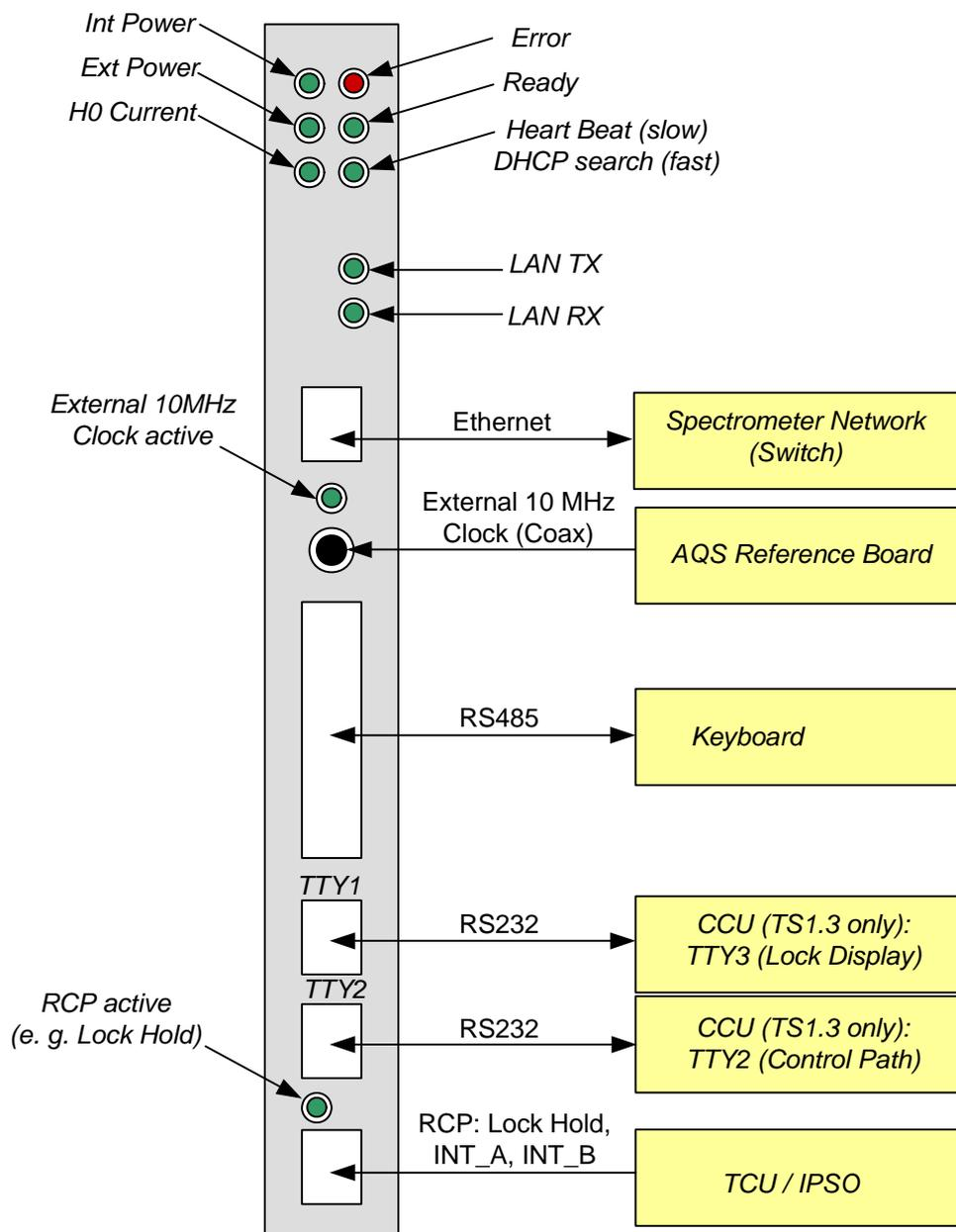
Figure 10.1 ELCB front panel with LED's and connectors
