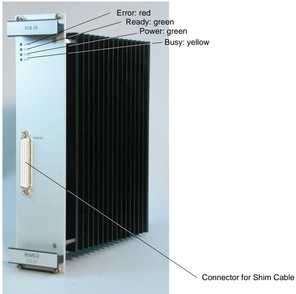
Figure 11.6 The picture below shows a SCB20 shim current board
