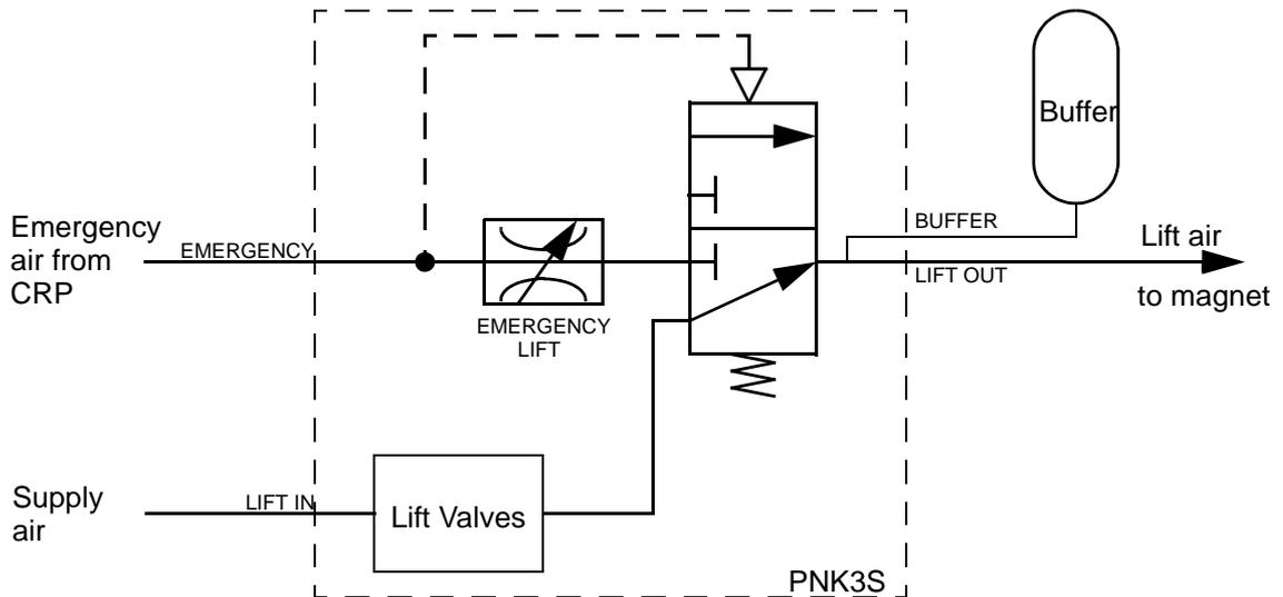
Figure 15.7 Block Diagram Emergency Lift
