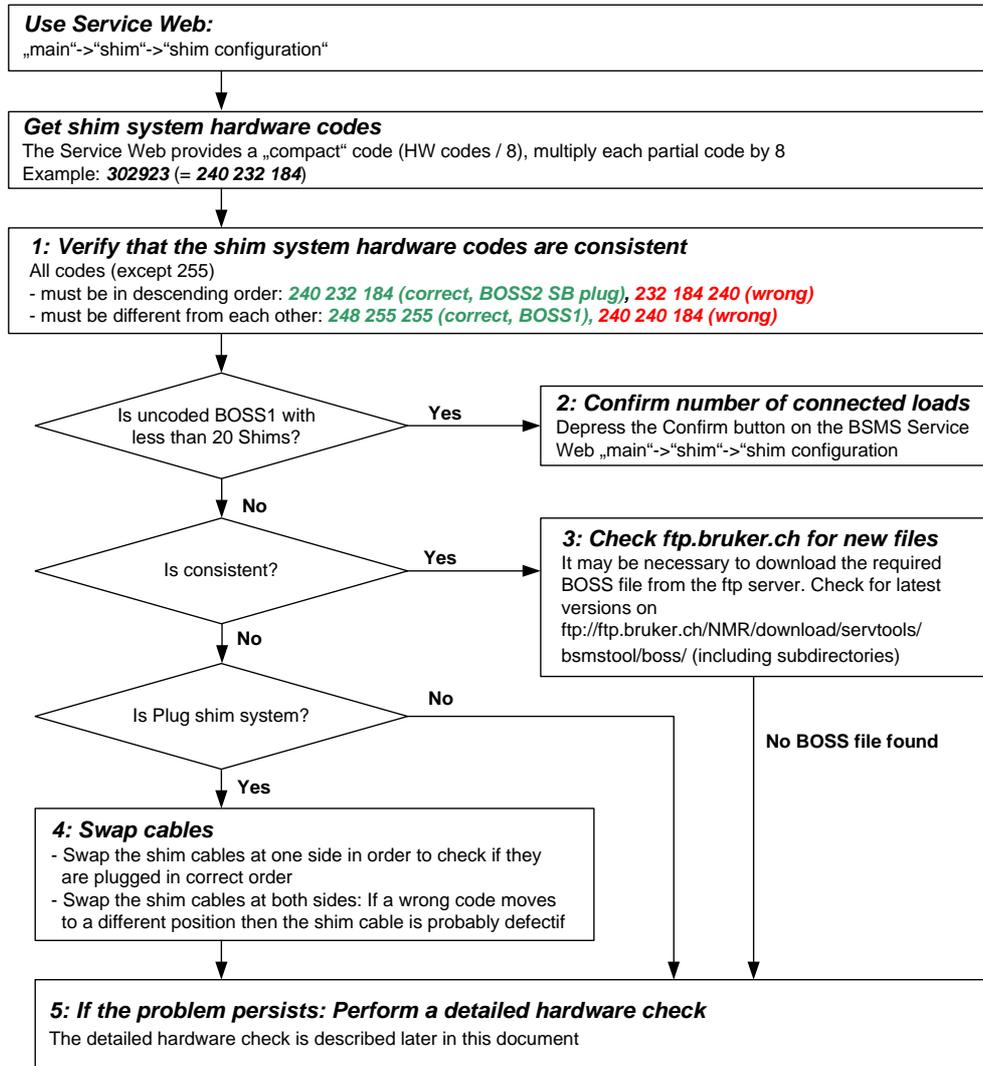
Figure 11.12 Troubleshooting problems with Shim System and BOSS file
