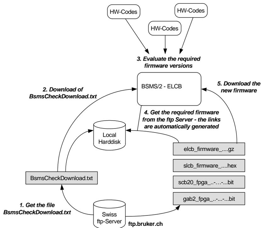
Figure 6.1 Principle of firmware upgrading
