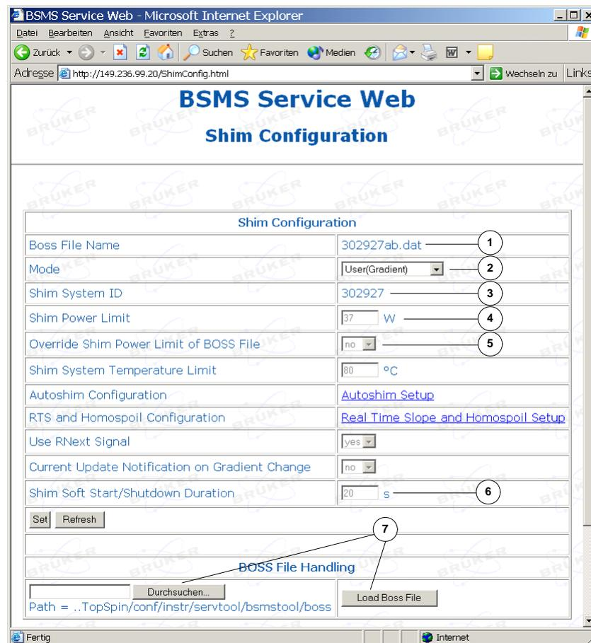
Figure 11.9 Setup and Configuration of the Shim Subsystem
