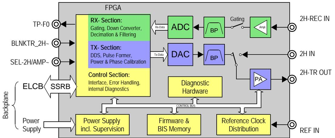
Figure 13.3 Block Diagram L-TRX unit
