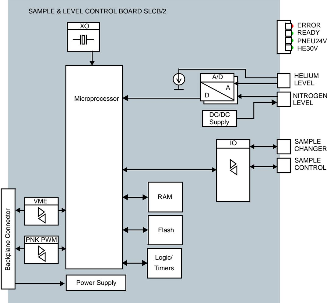
Figure 14.2 Block diagram of the SLCB/3
