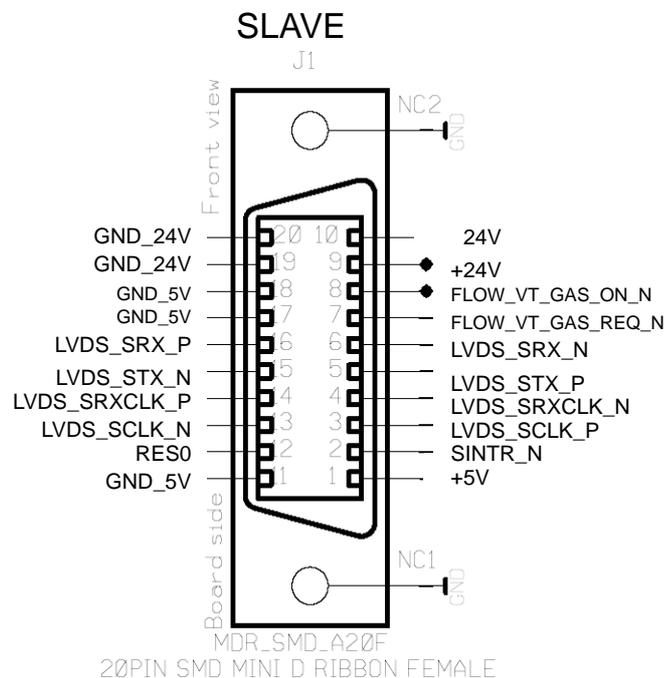
Figure 19.4 Slave pinning VPSB CTRL
