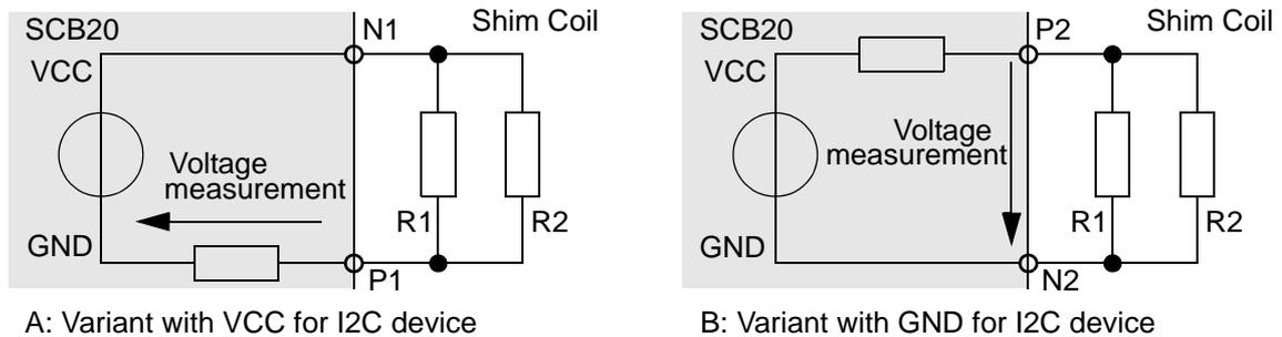
Figure 11.5 Interface for HW codes and I2C identification device
