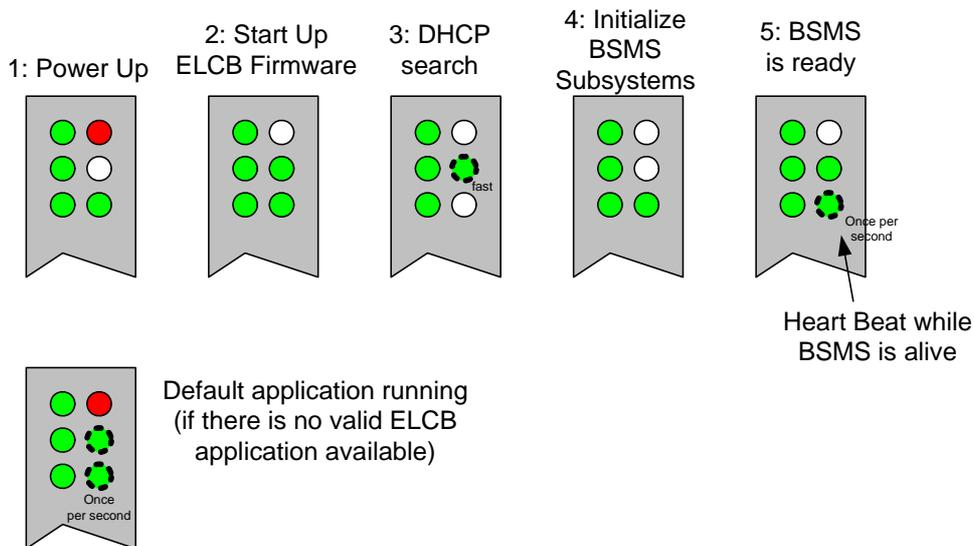
Figure 10.5 LED's indicating different states during start up
