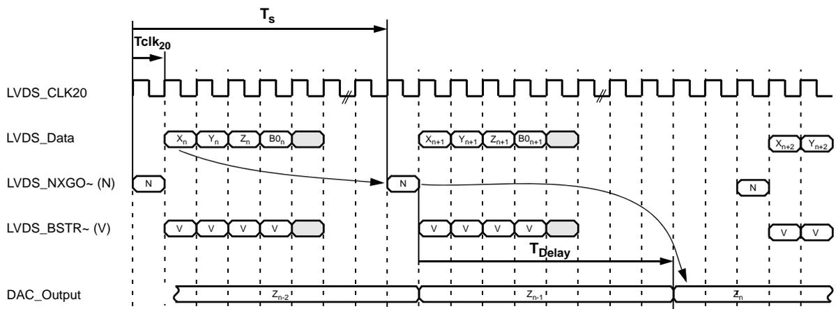
Figure 12.9 Timing for the communication over the 28 bit LVDS link
