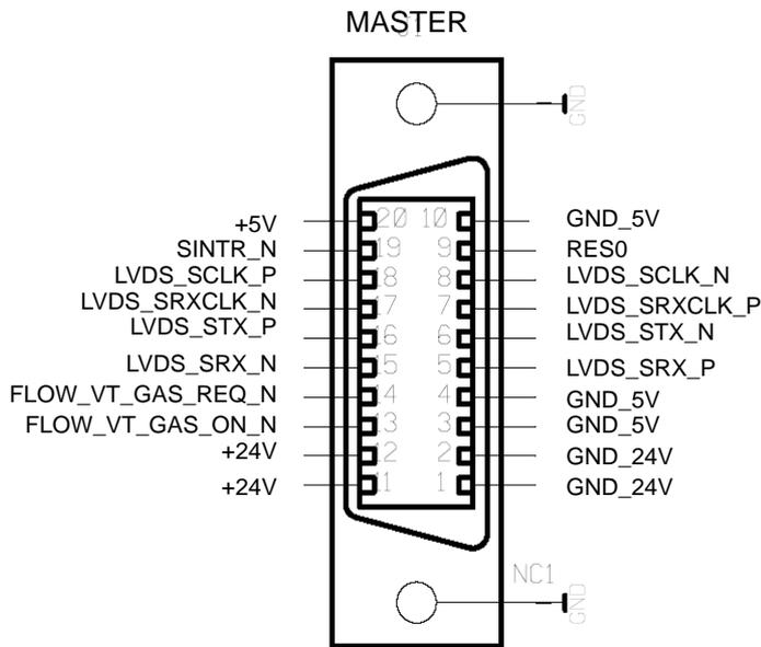
Figure 18.9 Pinning VPSB CTRL
