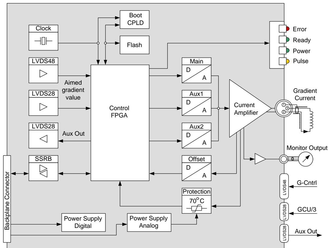
Figure 12.4 Block Diagram of the GAB/2 Gradient Amplifier board
