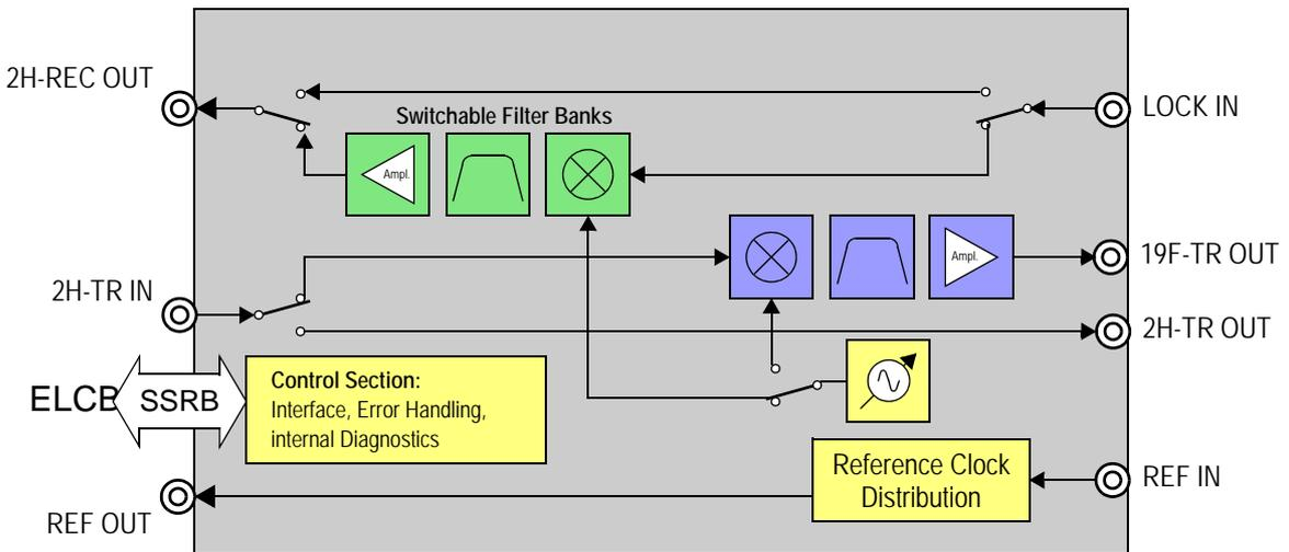
Figure 13.2 L-19F Block Diagram
