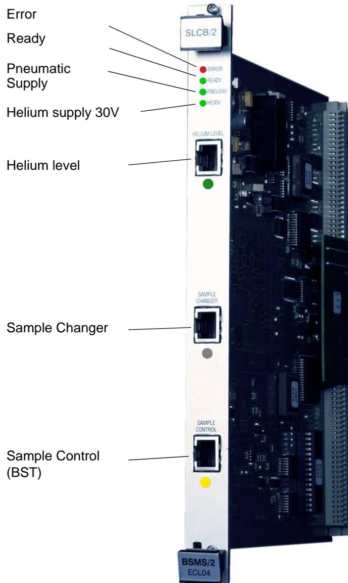
Figure 14.3 The picture below shows a SLCB/2
