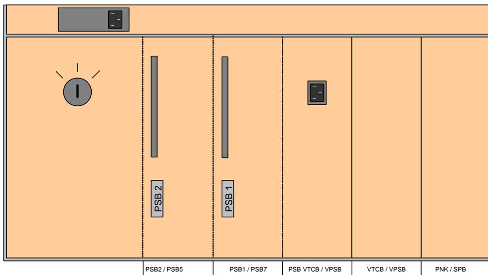
Figure 8.2 Power supplies for any non-L-TRX configuration (rear side)
