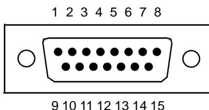
Figure 20.6 D-Sub 15 male, pin assignment
