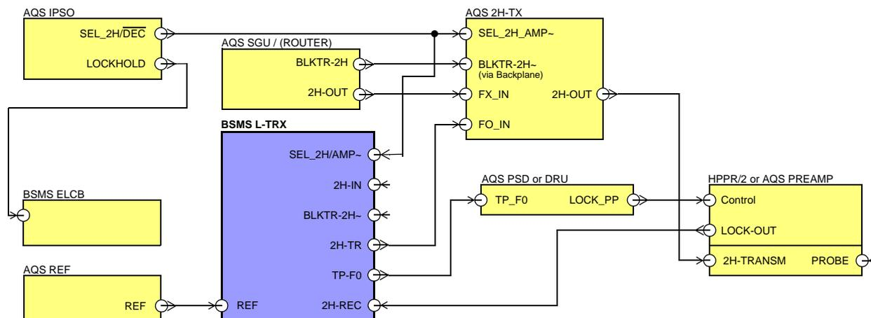
Figure 13.7 2H Lock system with additional, external 2H power amplifier
