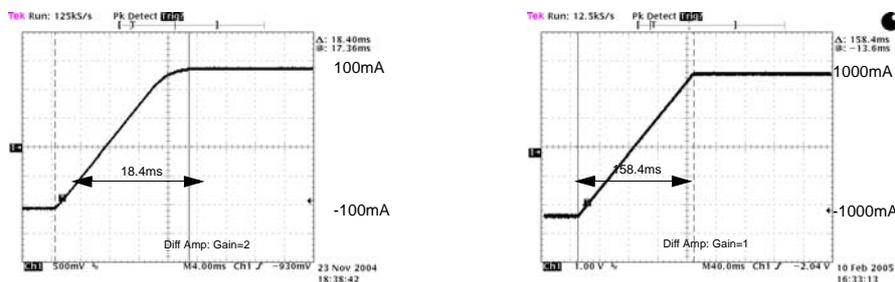
Figure 11.1 Step Response with step size of 200mA (left) and 2.0A (right)
