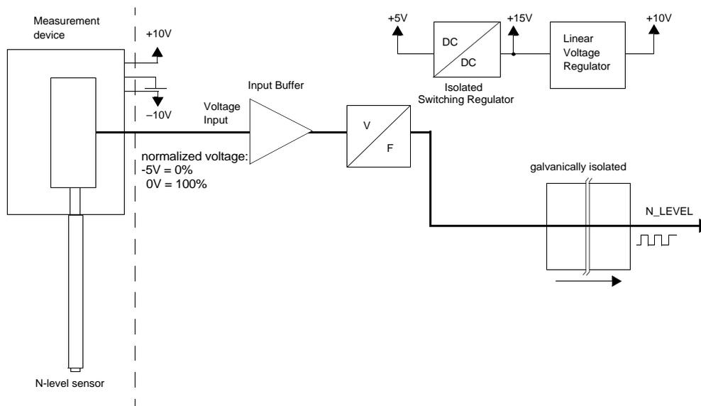
Figure 14.7 Analog nitrogen level measurement block diagram
