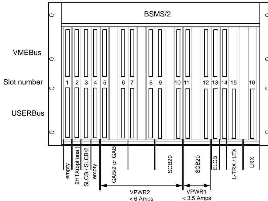
Figure 8.10 The BSMS/2 rack with the specific slots
