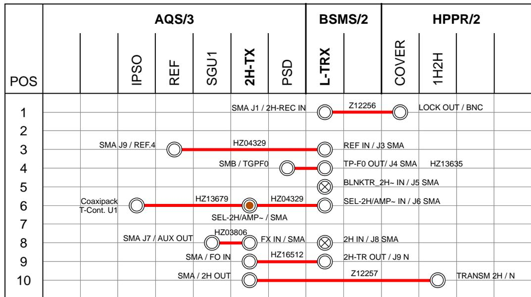
Additional requirements: ● SMA-T adapter (67072) ⊗ not used (BLNKTR\_2H- IN must be open!)
