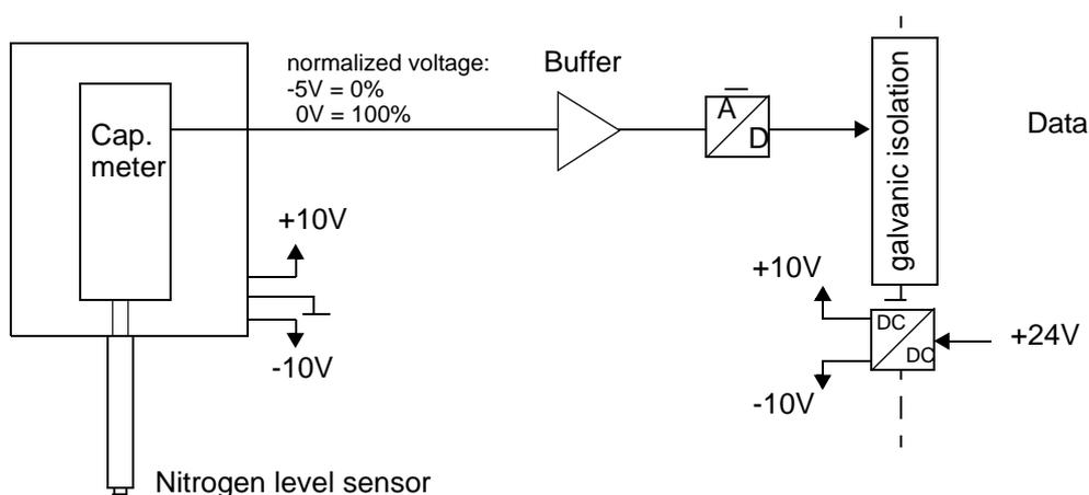
Figure 18.6 Analog nitrogen level measurement block diagram
