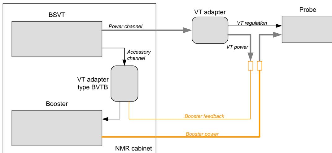
Figure 17.6 Booster in operation
