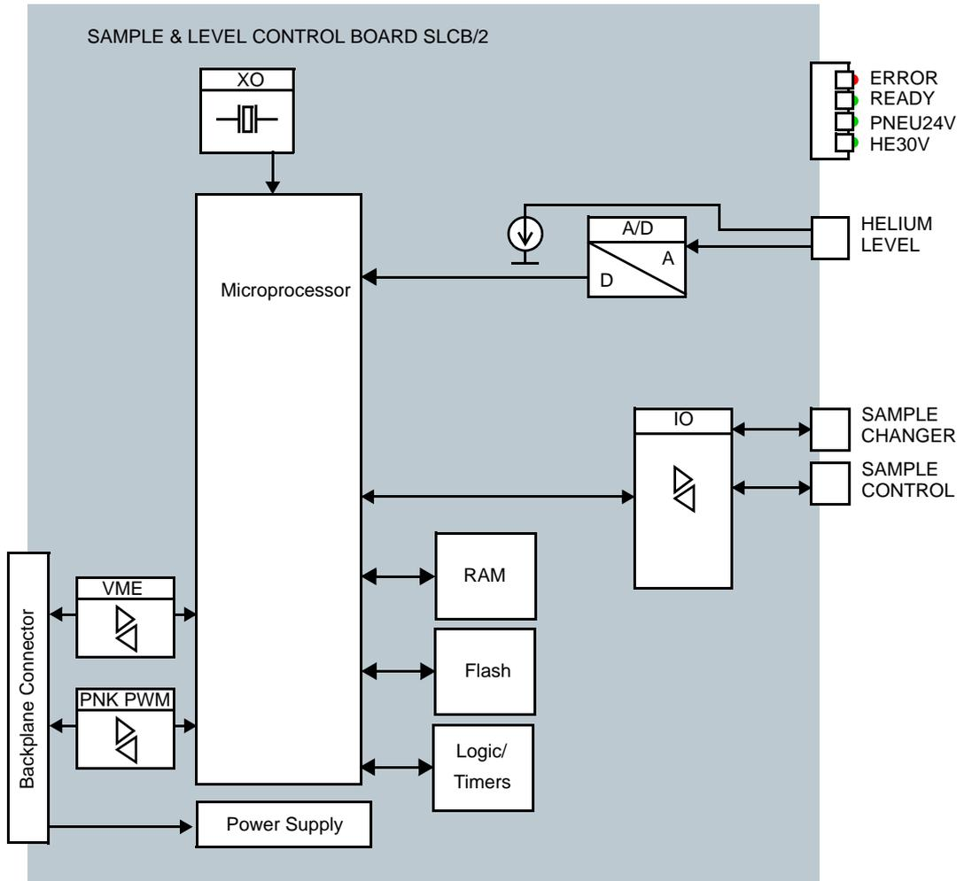
Figure 14.1 Block diagram of the SLCB/2
