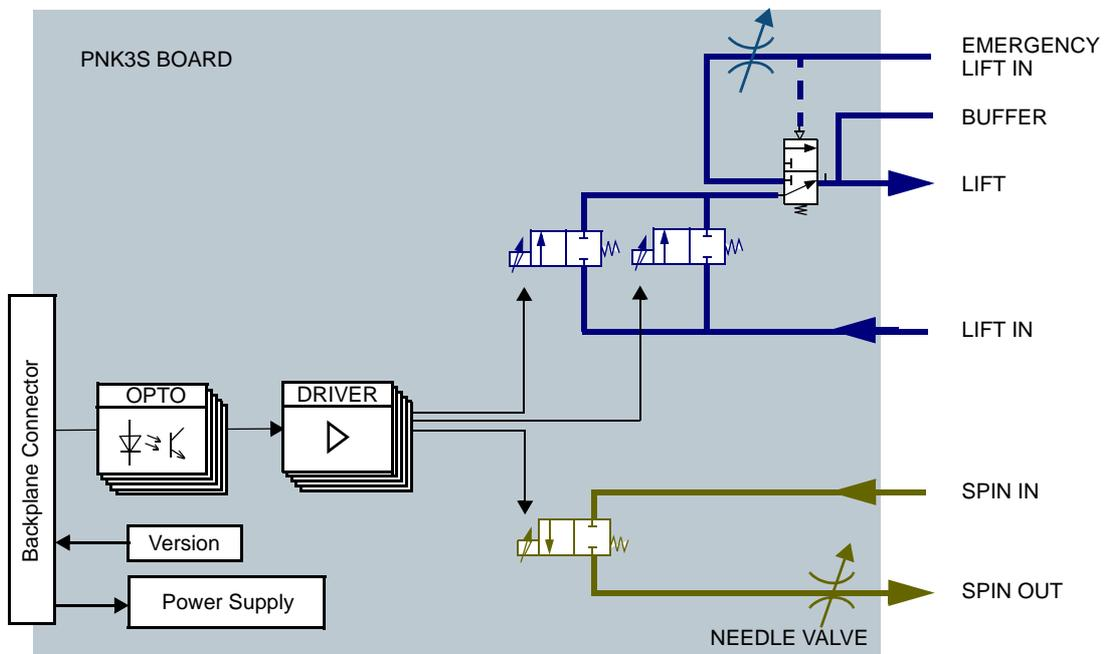
Figure 15.2 Block diagram of the PNK3S module
