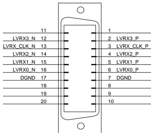
Figure 12.7 LVDS 28 interface used in AVII spectrometers
