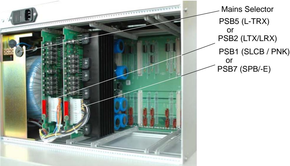
Figure 8.12 Rear View of BSMS/2 Rack
