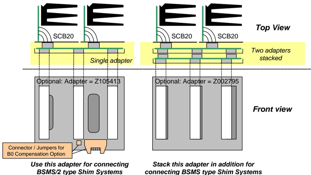
Figure 11.3 Adapter for BSMS/2 and Adapter stack for former BSMS
