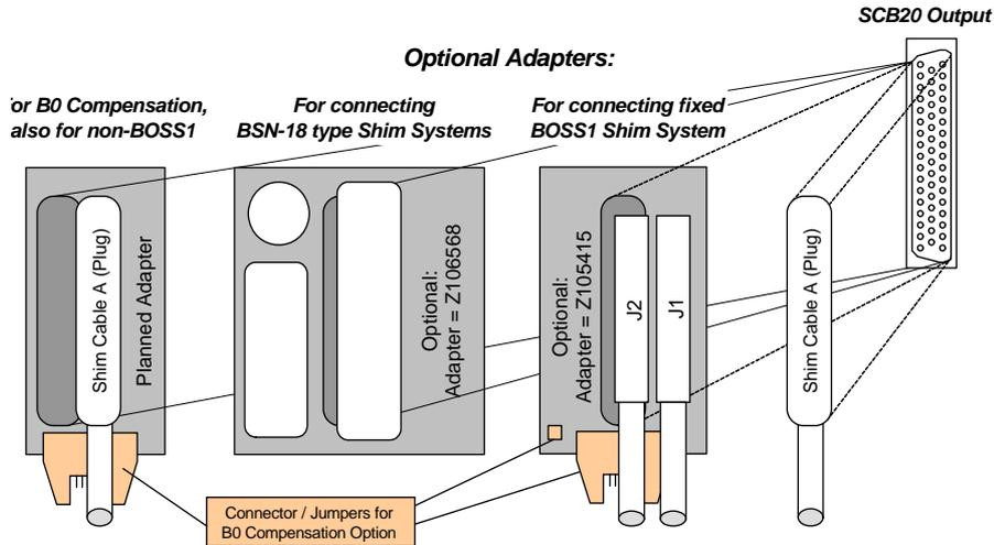
Figure 11.2 Adapters for BOSS1 and BSN-18 type Shim Systems
