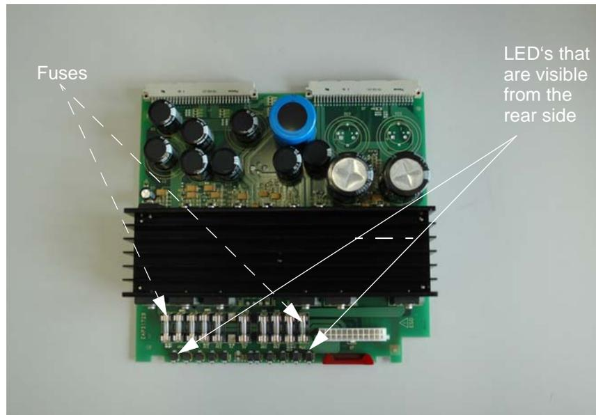
Figure 9.1 View of a PSB2 module
