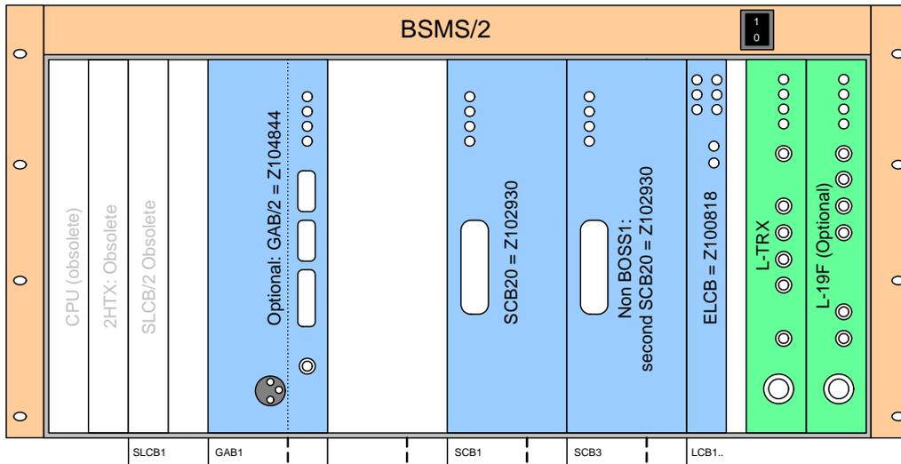
Figure 13.9 L-TRX and L-19F slots in BSMS/2 chassis (Front View)
