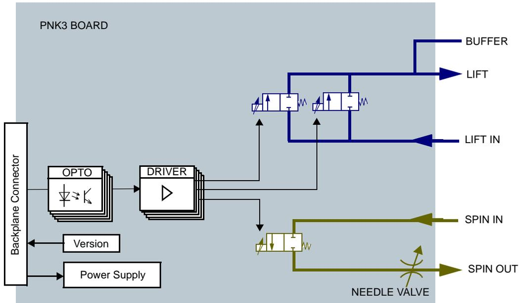
Figure 15.1 Block diagram of the PNK3 module
