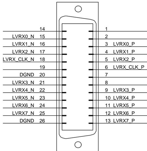
Figure 12.6 LVDS 48 interface used in AVANCE spectrometers with IPSO
