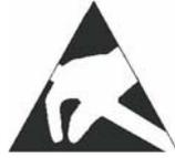
The packaging contains components which are sensitive to an electrostatic charge.
