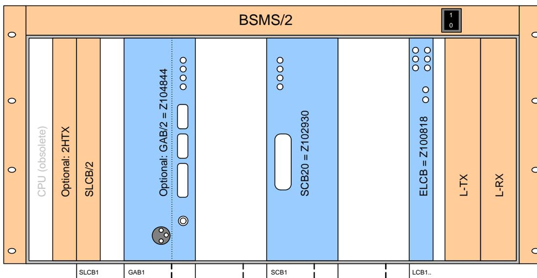
Figure 8.1 BOSS1 configuration with LTX / LRX (front)
