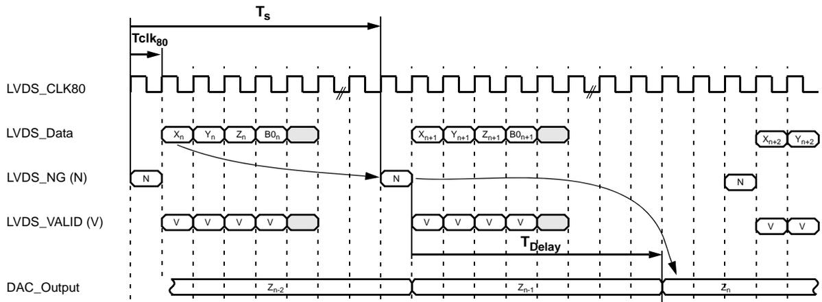
Figure 12.8 Timing for the communication over the 48 bit LVDS link
