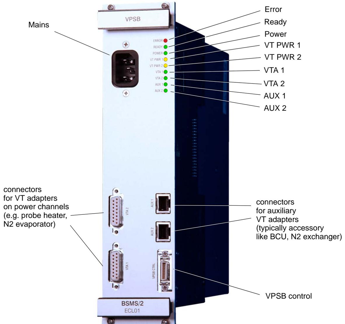
Figure 19.5 Front view of a VPSB
