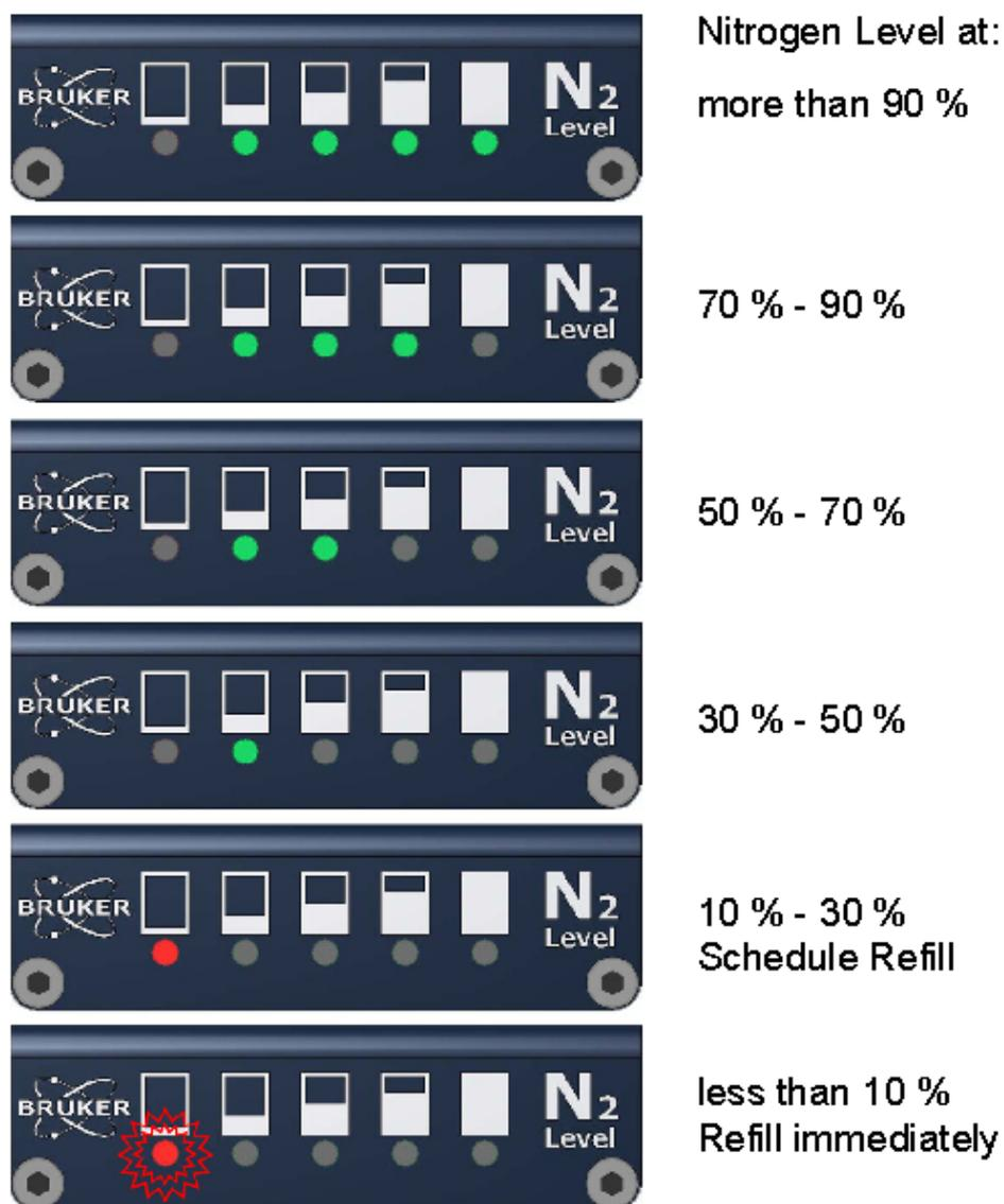
Figure 21.4 LED Code on N<sub>2</sub> level sensor
