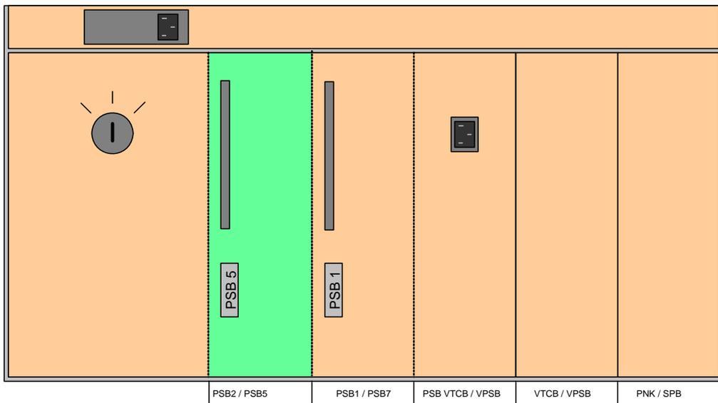
Figure 8.6 Power supplies for L-TRX (rear side)
