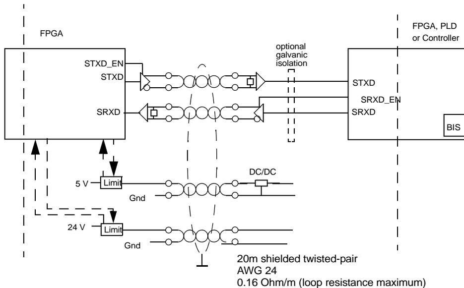
Figure 19.3 Overview Auxiliary Bus Connector
