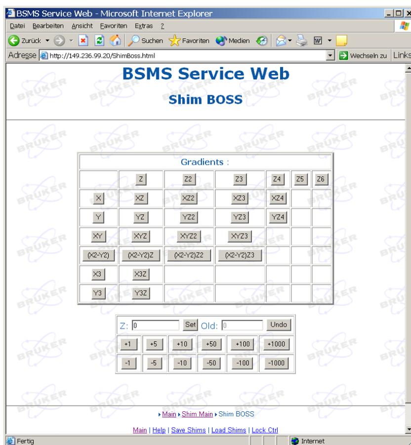
Figure 11.10 View and manual modification of the Shims
