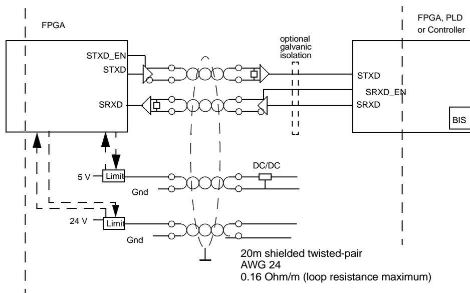
Figure 18.10 Overview Auxiliary Bus Connector (SPB-E) only
