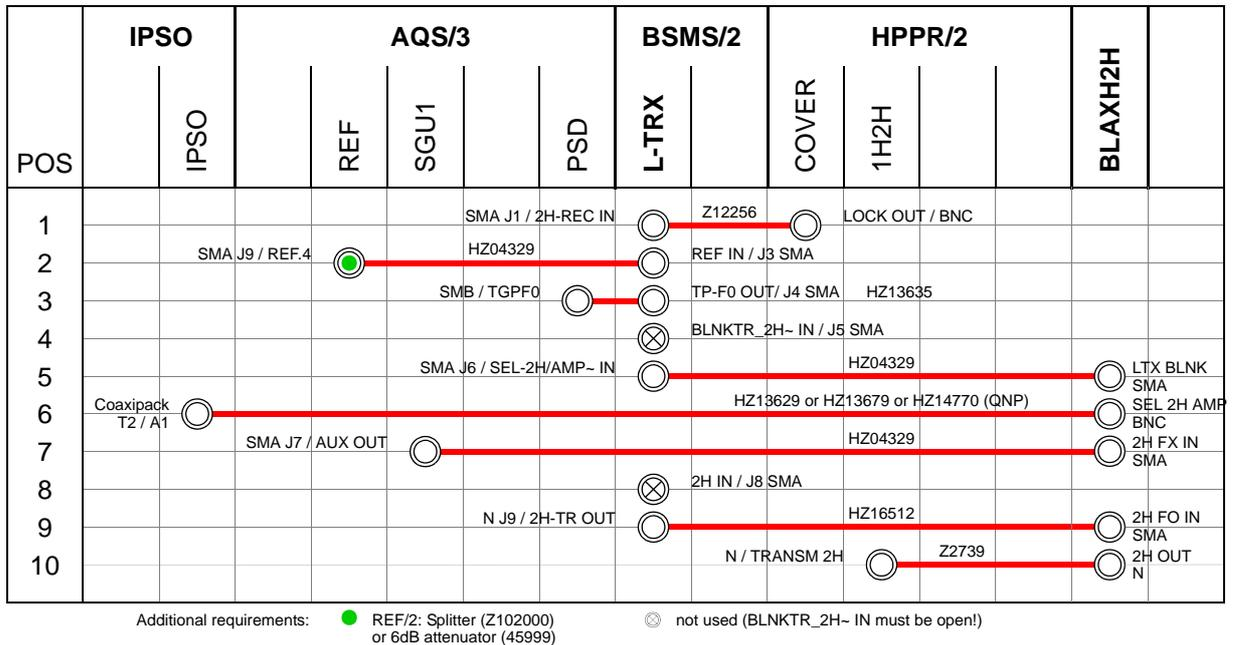
Figure 13.14 Wiring AVANCE III One & TwoBay with BLAXH2H (H14008, H14010 and one of H14014 or H14015 or H14016)
