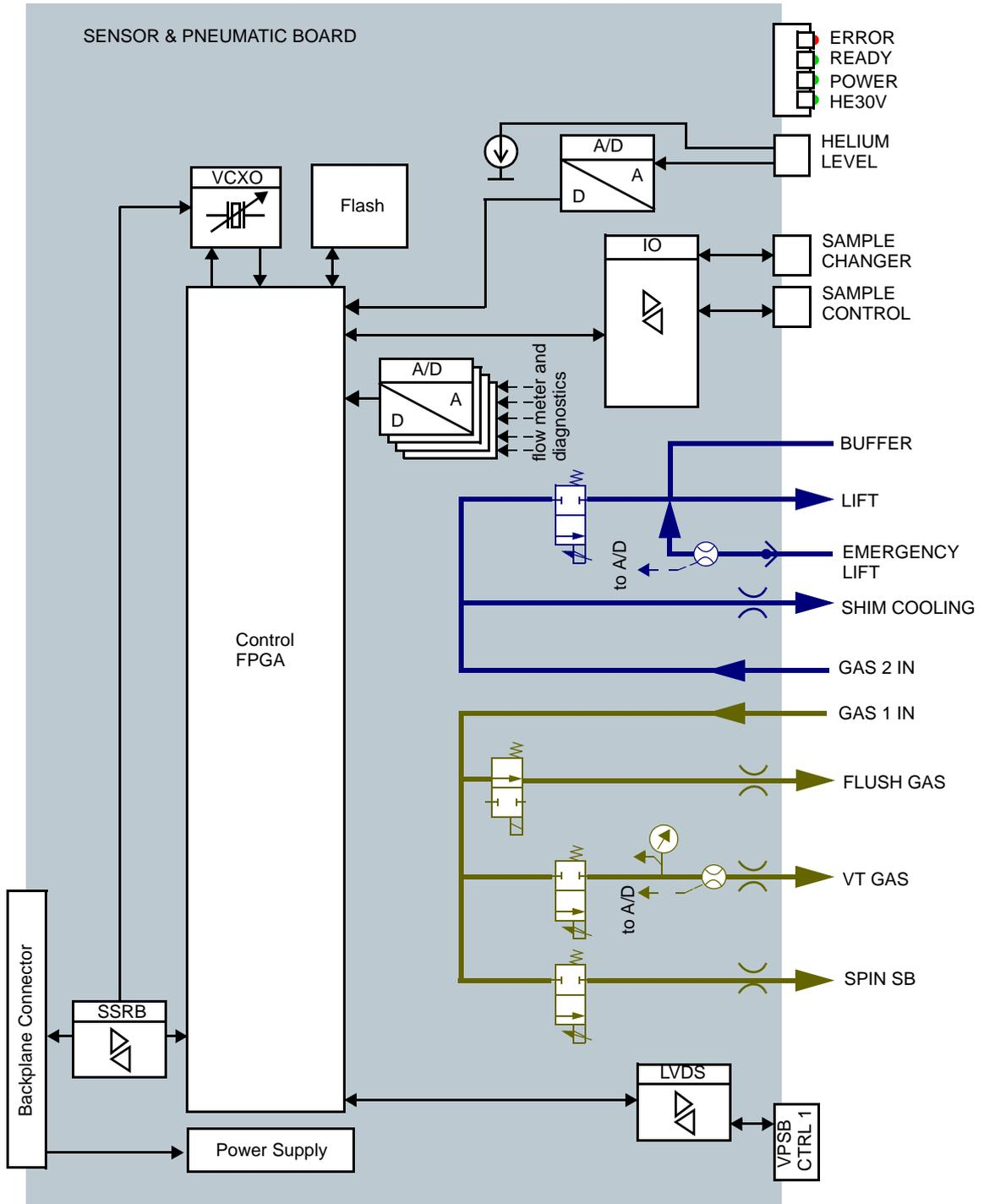
Figure 18.1 Block diagram of the SPB
