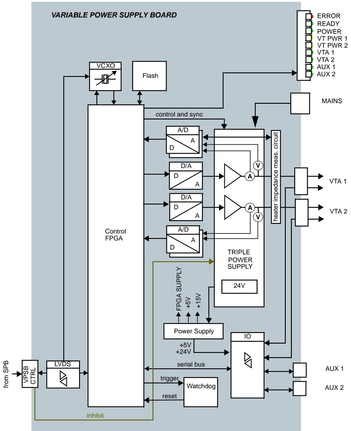
Figure 19.1 Block diagram of the VPSB
