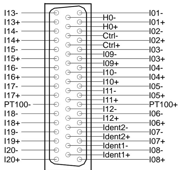
Figure 11.7 Pinout of the 50 pin Shim connector
