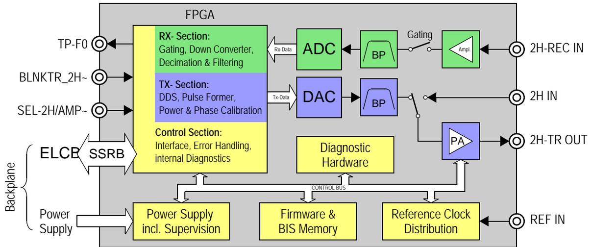
Figure 13.1 L-TRX Block Diagram
