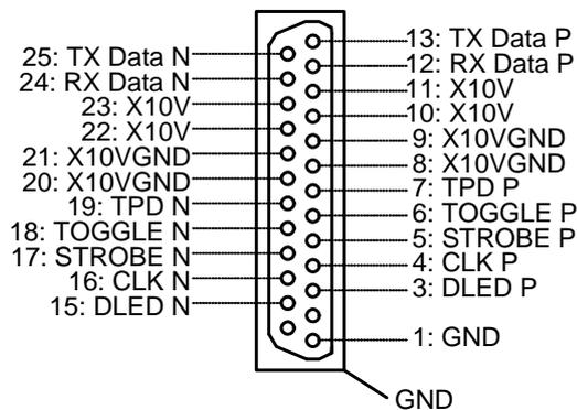
Figure 10.7 DSUB-25 connector for keyboard
