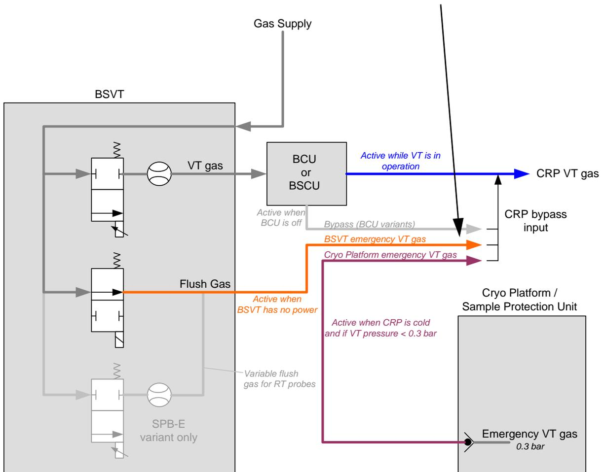
Figure 17.2 VT emergency gas flow
