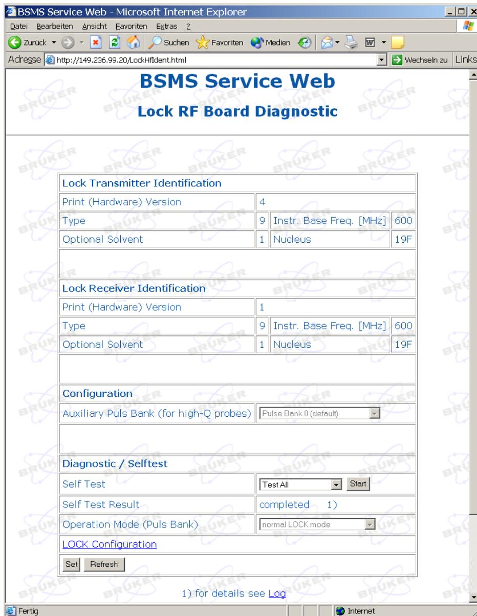
Figure 10.11 Lock RF boards - information and diagnostics
