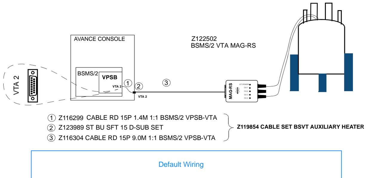
Figure 22.1 Connection to BSMS/2 (Monitoring and Service)
