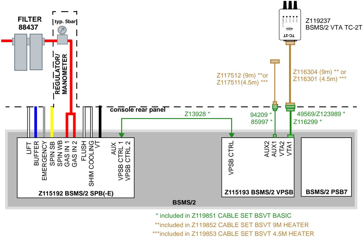
Figure 16.7 Basic BSMS/2 configuration with VT system option
