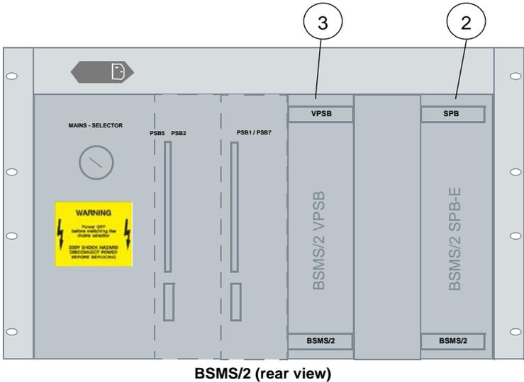
Figure 16.6 BSMS/2 units that support nitrogen level sensors
