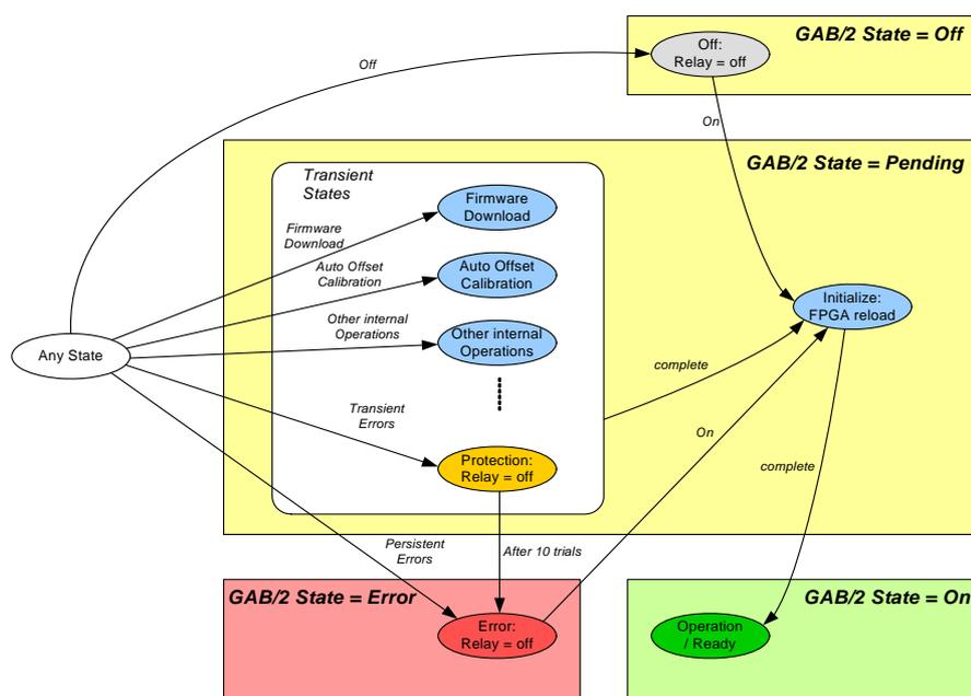
Figure 12.5 The GAB/2 Control State Machine
