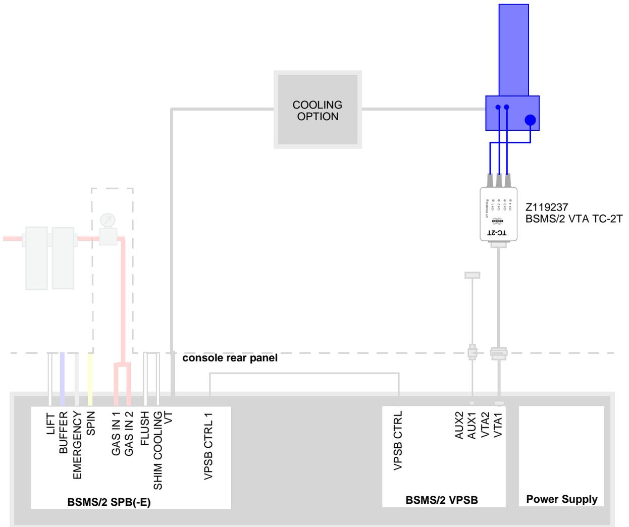
Figure 16.11 Solids probehead DVT with 2 thermocouple T
