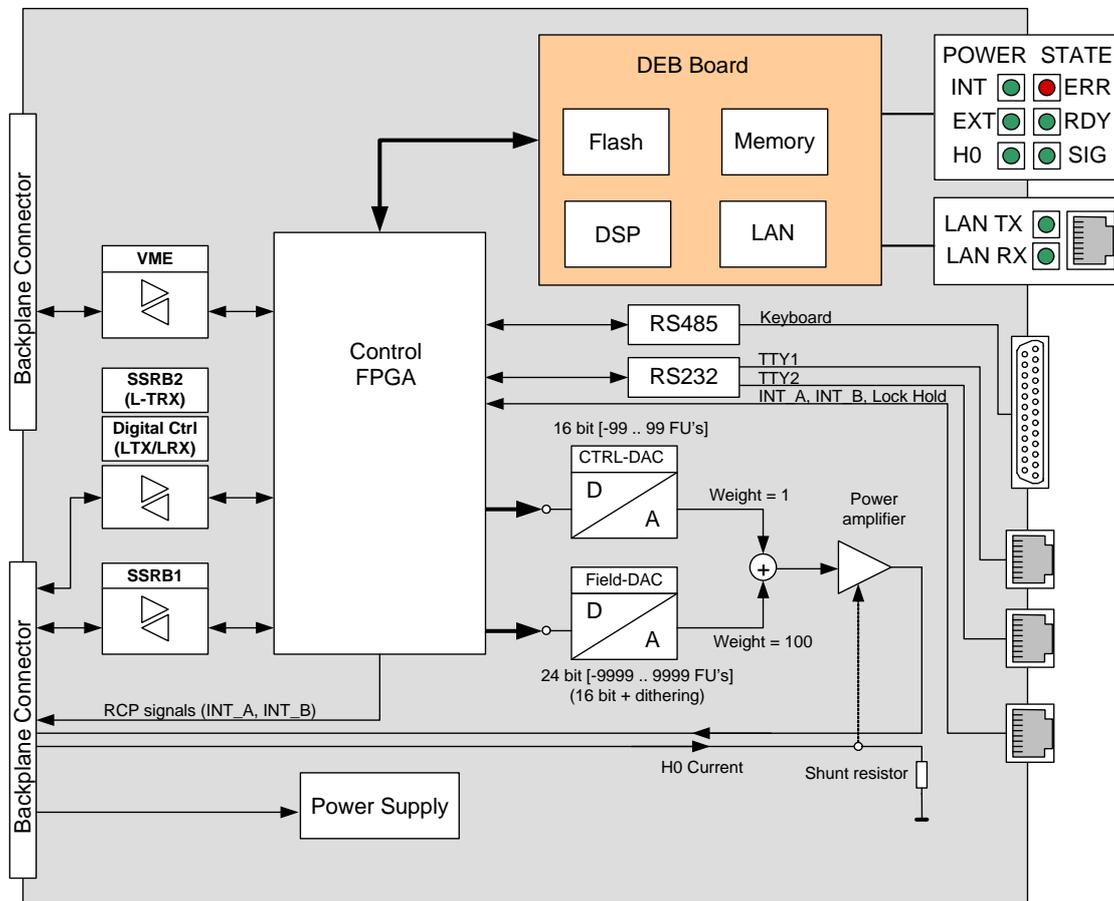
Figure 10.2 Functional system architecture
