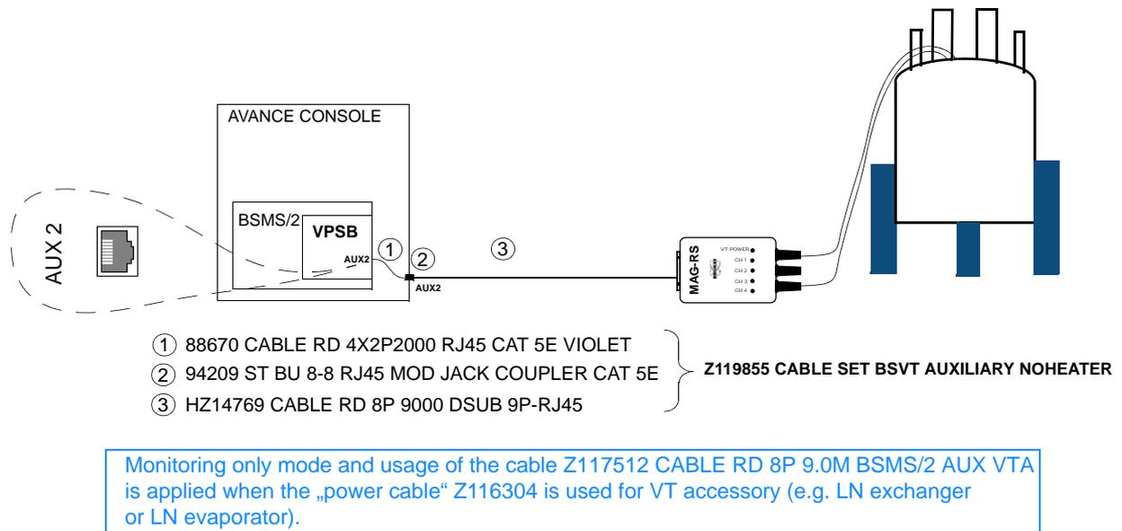
Figure 22.2 Connection to BSMS/2 (Monitoring only)
