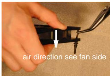
3) place the fan wire side towards the solder pads
