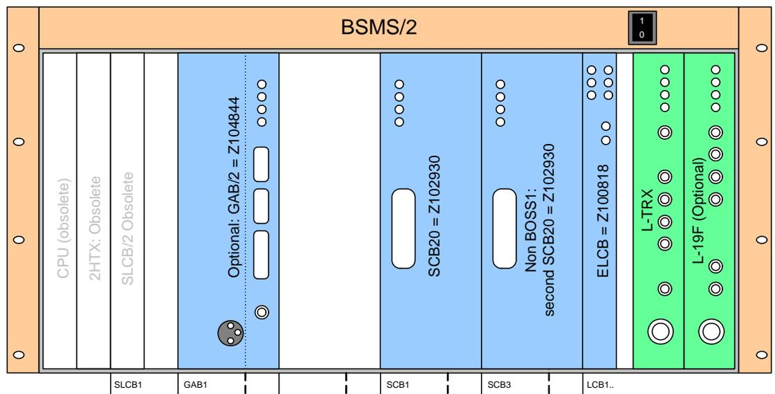
Figure 8.7 Configuration with L-TRX and optional L-19F unit (example with GAB/2)
