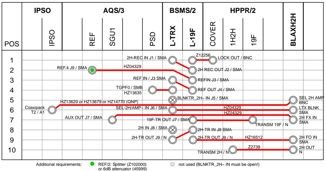
Figure 13.15 Wiring AVANCE III One & TwoBay with L-19F and BLAXH2H (H14008, H14010, Z125188 and one of H14014 or H14015 or H14016)
