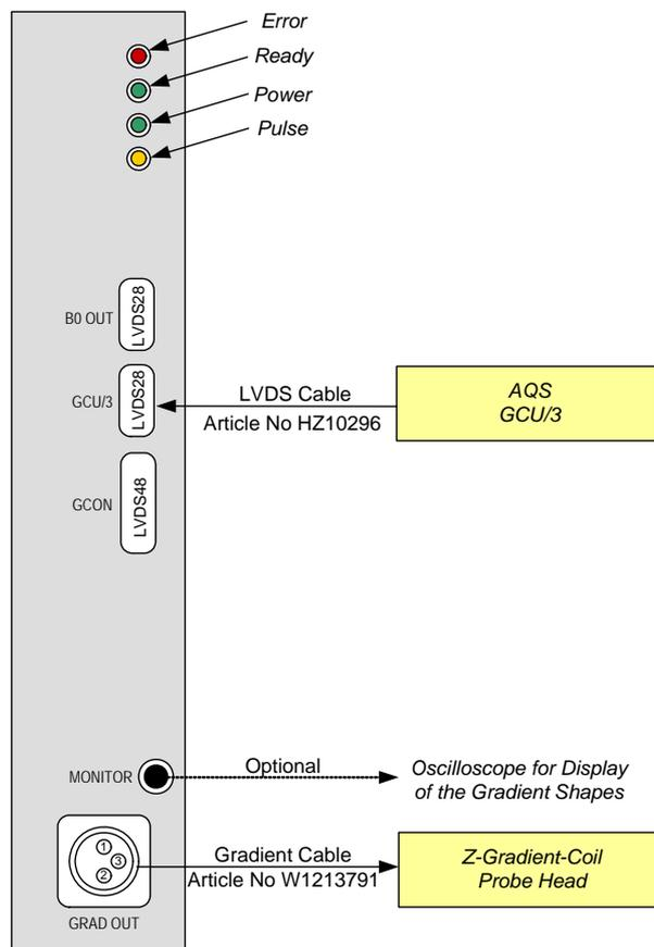
Figure 12.1 GAB/2 in an AVII spectrometer
