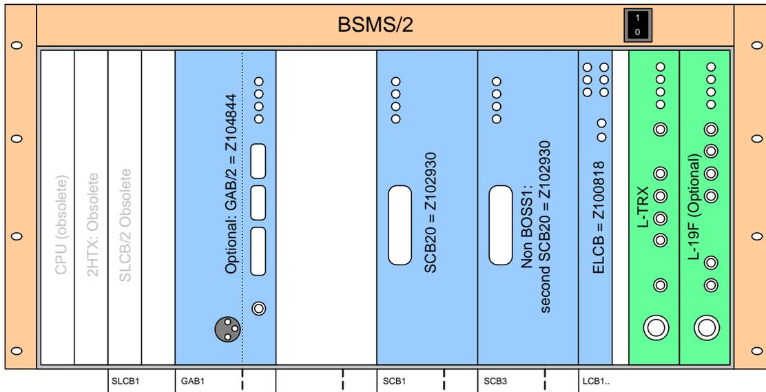
Figure 8.5 Configuration with L-TRX (example with GAB/2)
