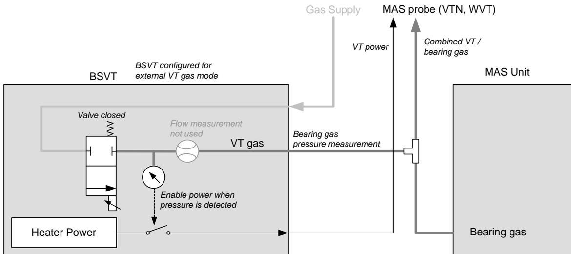
Figure 17.4 External VT gas supply (e. g. MAS bearing gas)
