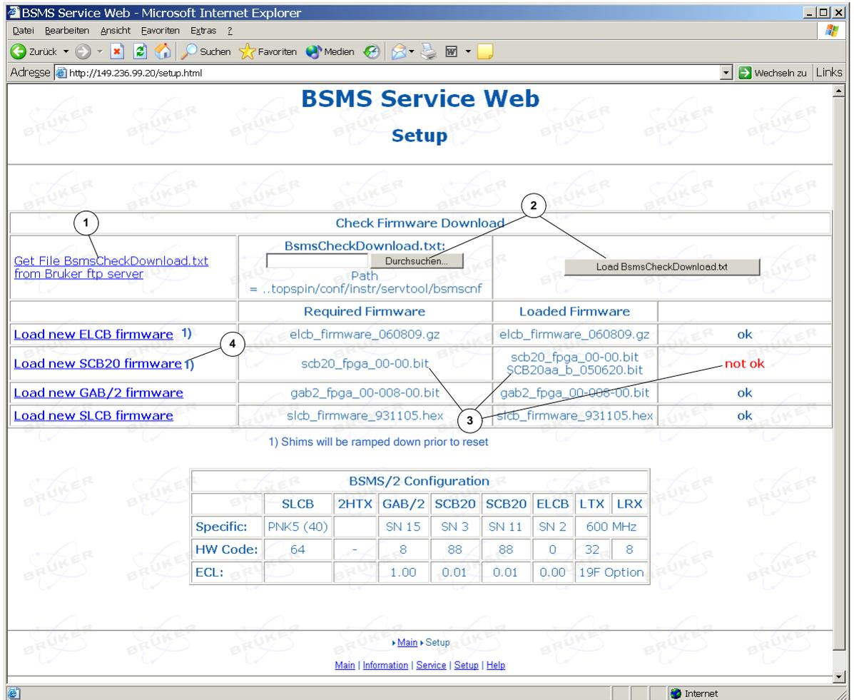
Figure 6.2 Setup of the BSMS/2 firmware
