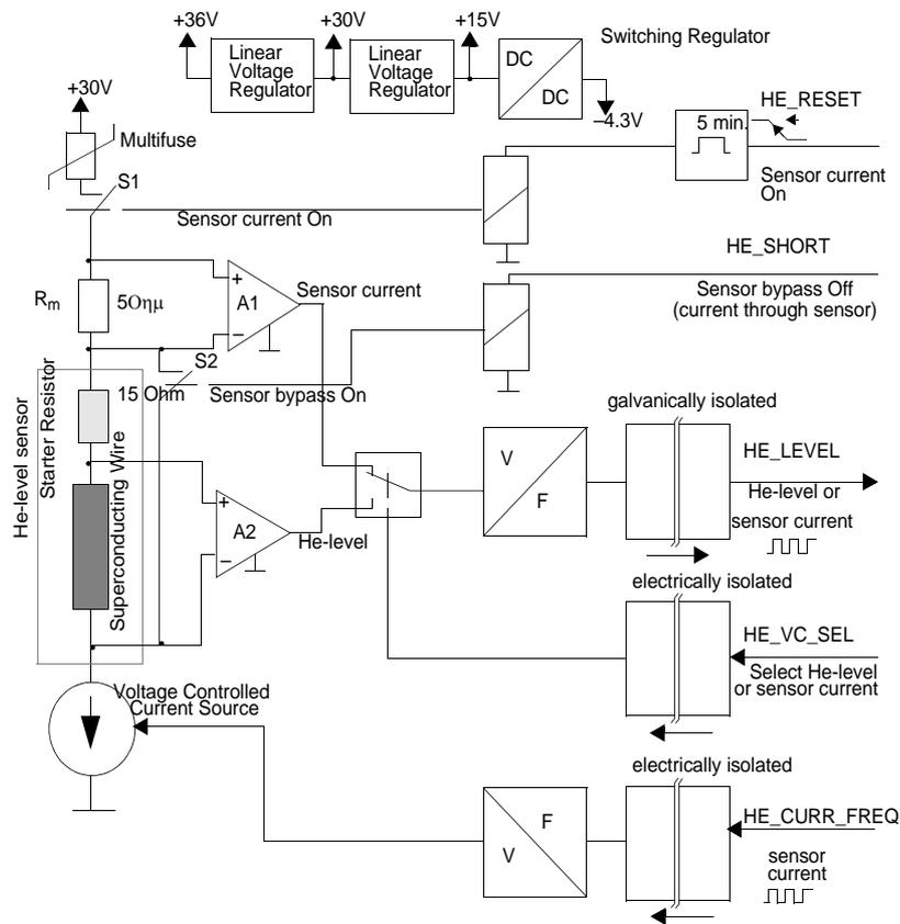
Figure 14.5 Block diagram Helium level measurement
