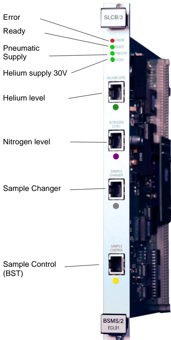
Figure 14.4 The picture below shows a SLCB/3
