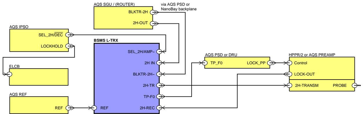
Figure 13.5 2H Lock system with L-TRX internal power amplifier for gradient shimming
