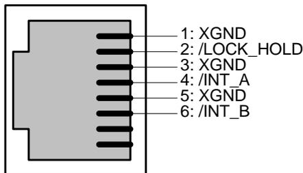
Figure 10.6 RJ45 connector for real time control
