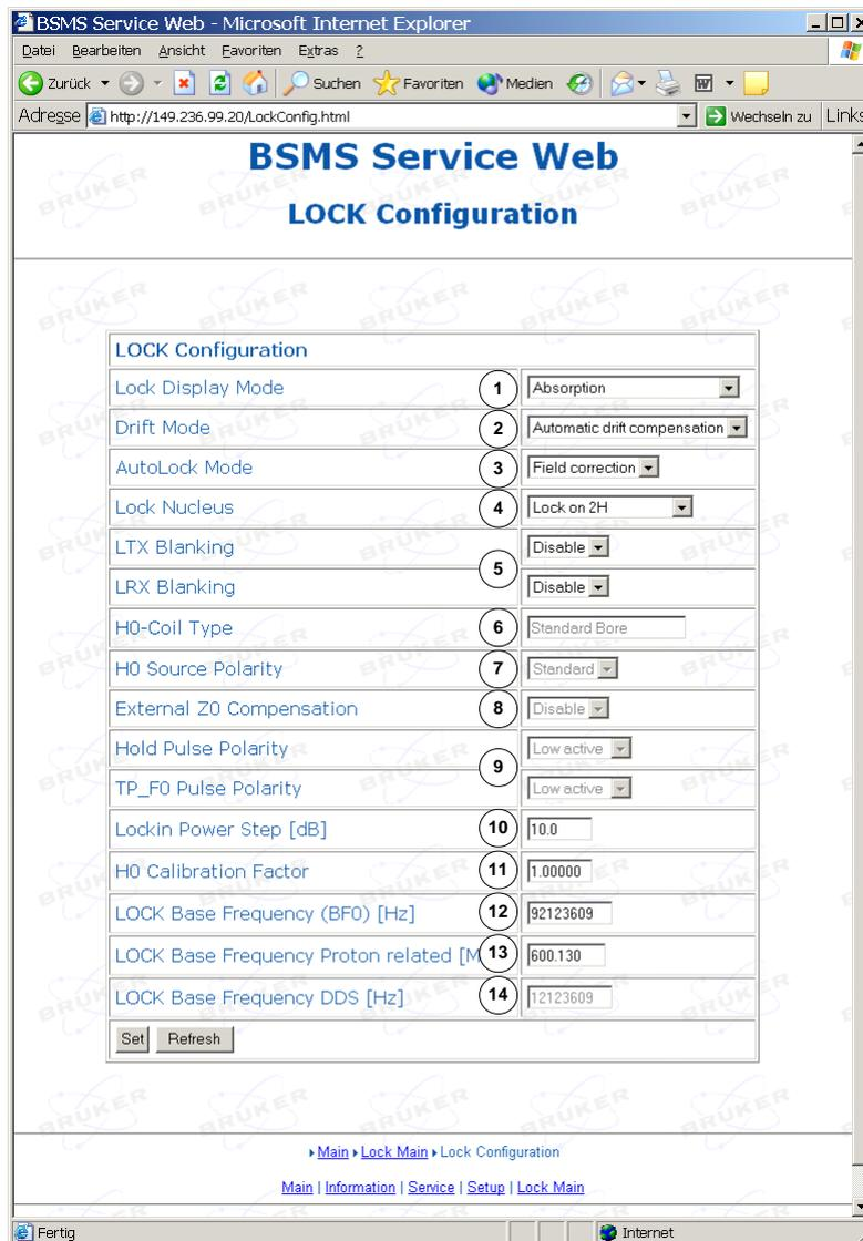
Figure 10.10 Configuration of NMR lock
