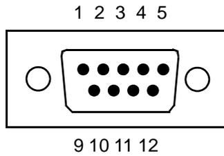
Figure 21.5 D-Sub 9 male, pin assignment
