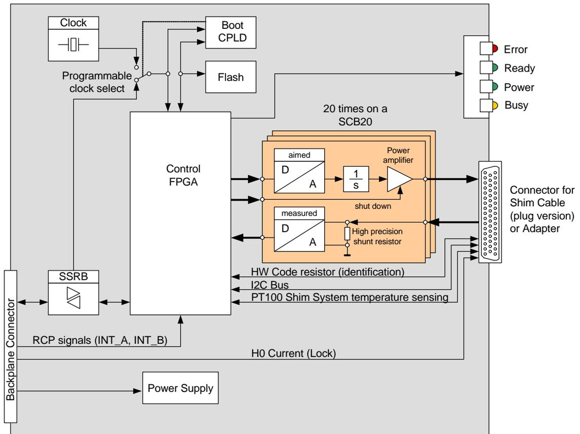
Figure 11.4 Block Diagram of the SCB20 shim current board
