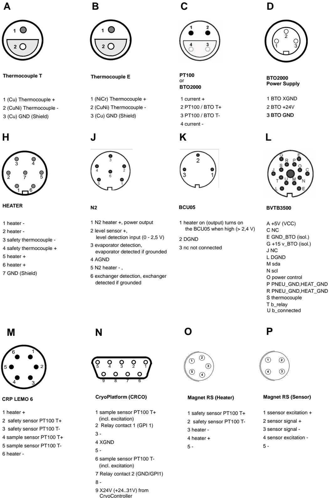
Figure 20.1 VTA cable connectors
