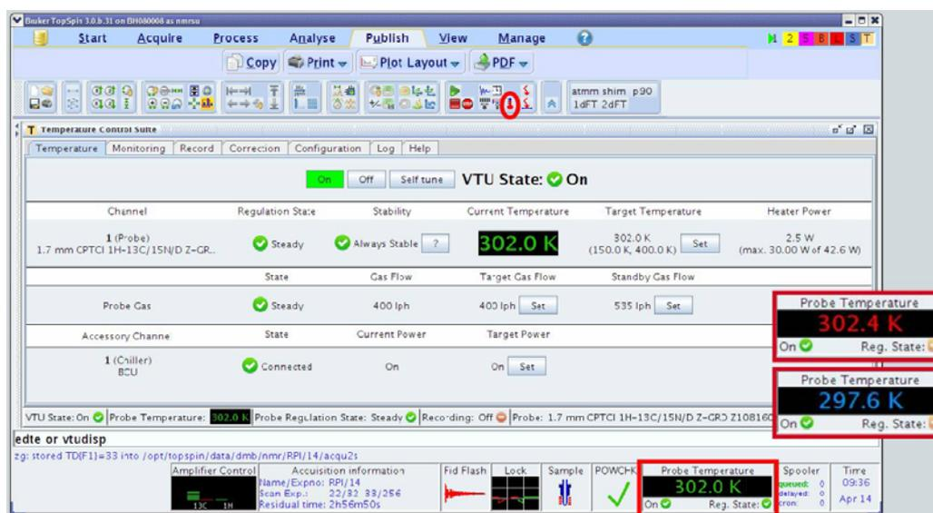
Figure 16.3 Example of the VT panel within Topspin3.0
