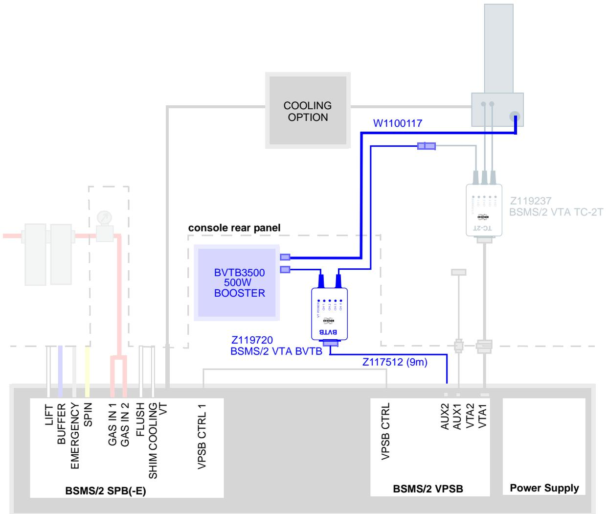
Figure 16.13 Power booster and solids probehead
