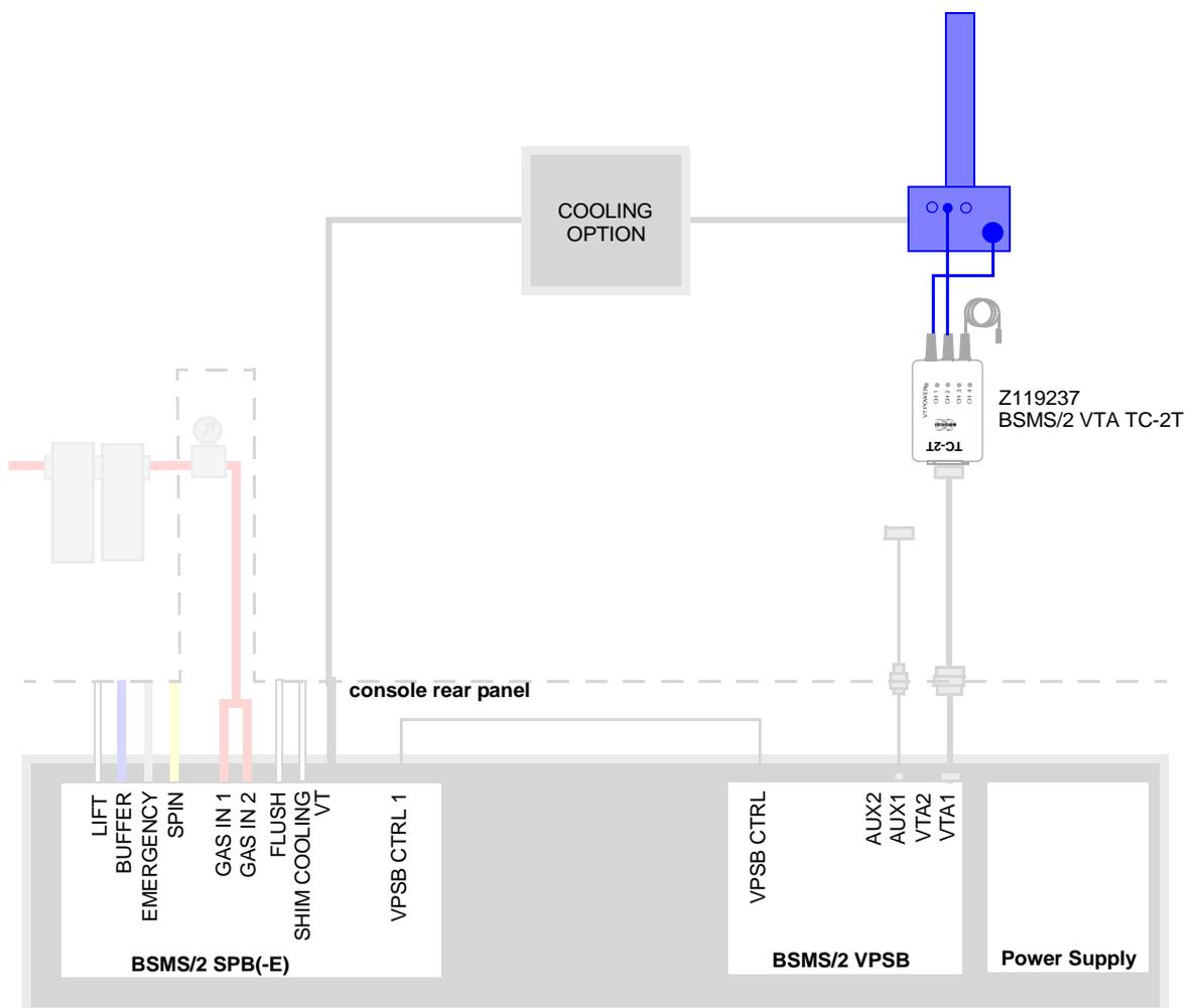
Figure 16.8 Standard HR RT probe with thermocouple T
