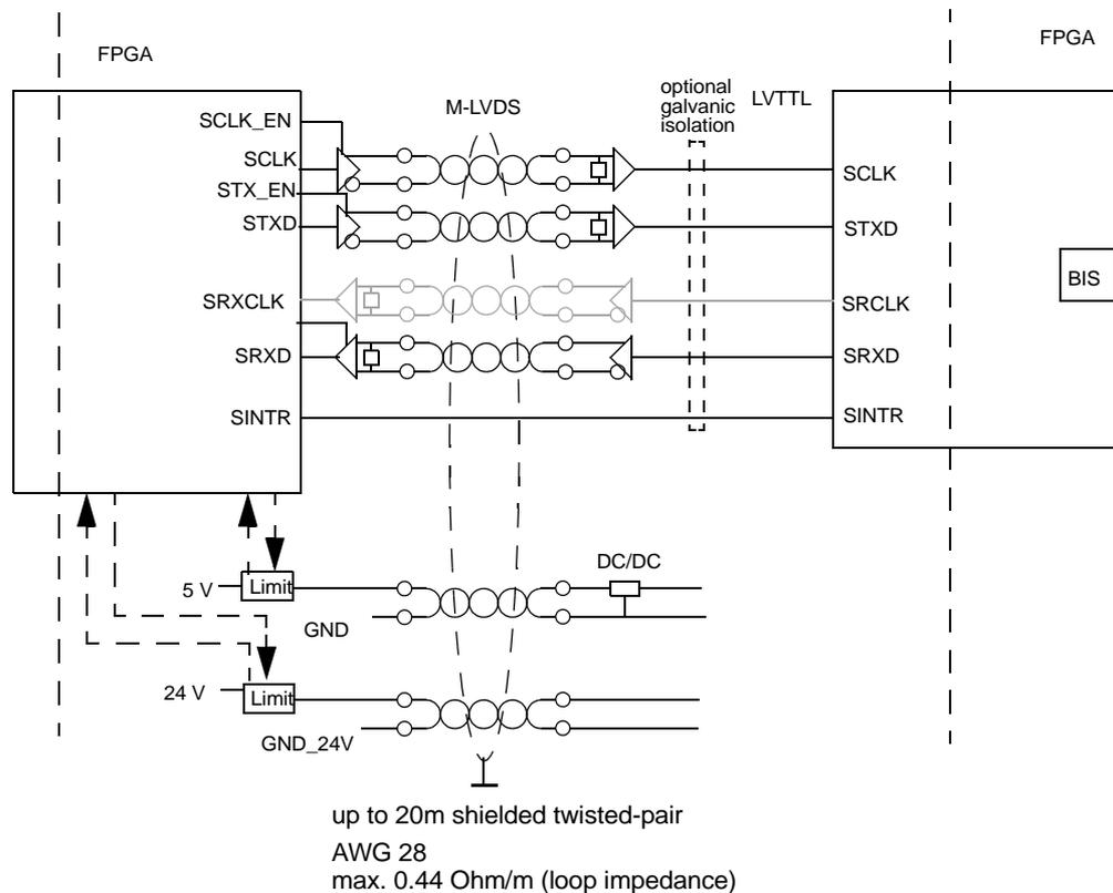
Figure 18.8 Overview of point-to-point full duplex VPSB CTRL interface
