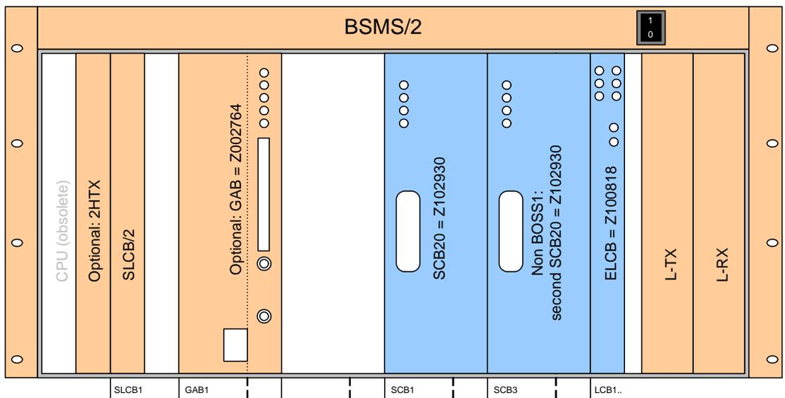
Figure 8.4 AVANCE II - configurations with GAB
