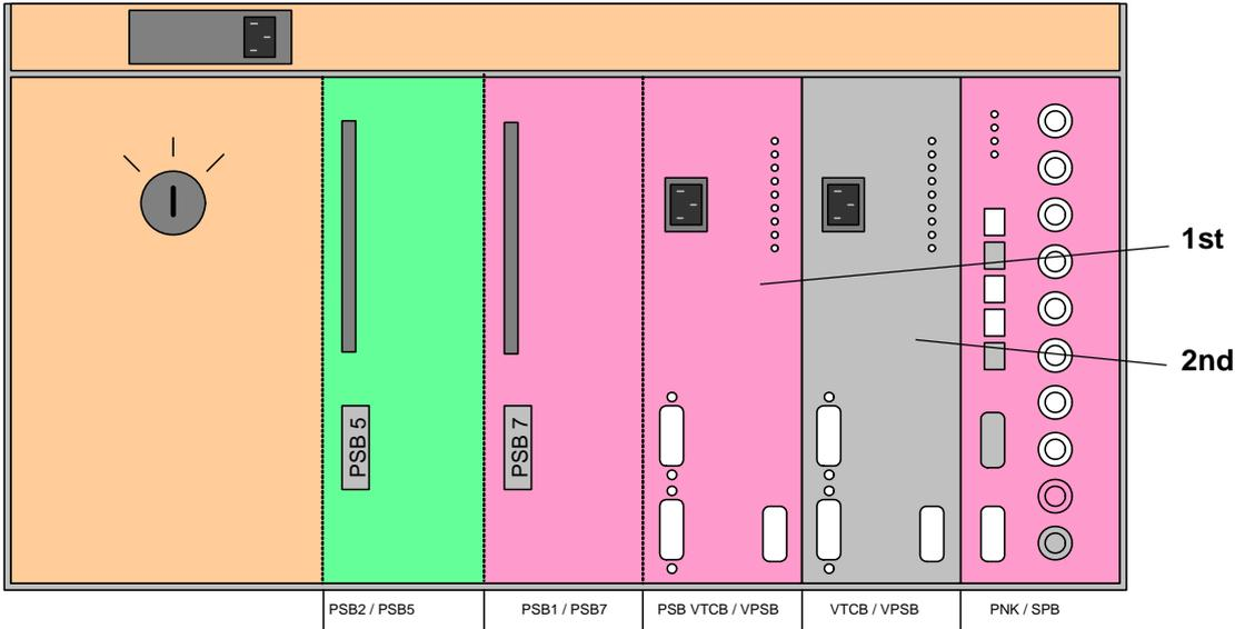
Figure 8.8 SPB(-E), VPSB(s) and power supply (rear side)
