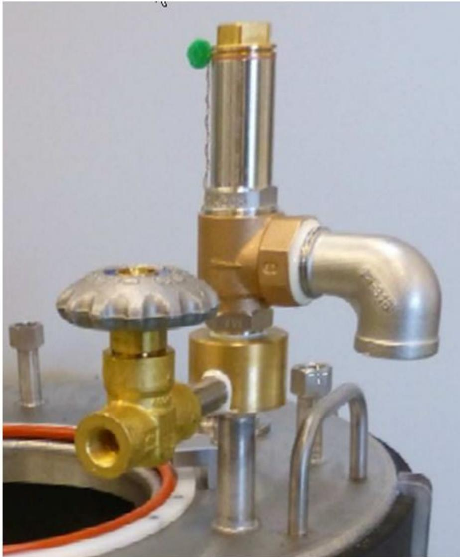
*Figure 13.2: Manual Reservoir Venting Valve*
