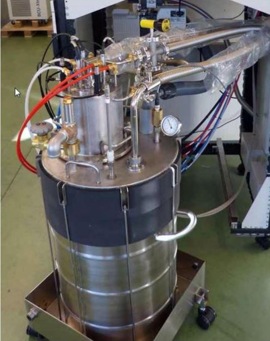
Figure 8.4: Exchanger Assembly with LN2 Reservoir
