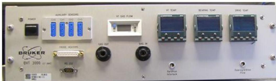
Figure 7.3: BVT3000 LT-MAS Front Panel
