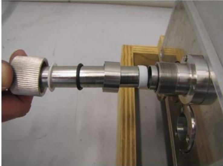
Figure 8.7: Connexion of Return Gas Line on Probe
