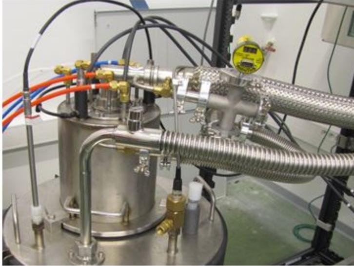
*Figure 8.5: Gas Return Line Installed*
