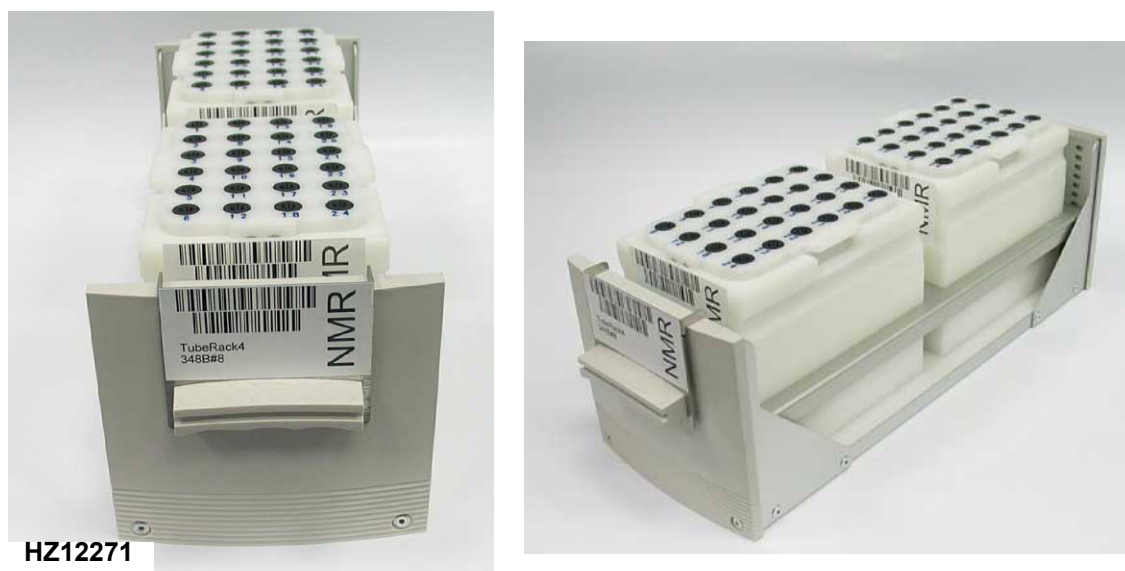
Figure 2.1: MATCH Tube Block with 1.0 mm Rack Front View (left), Top View (right)
