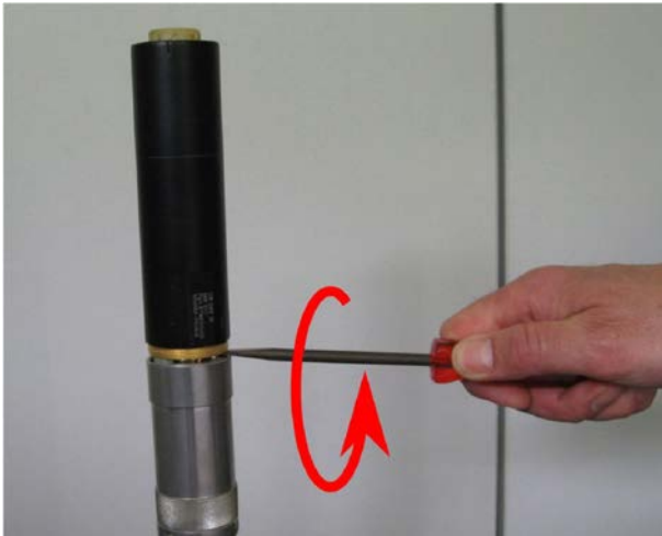
Figure 11.1: Gradient Coil Removal
