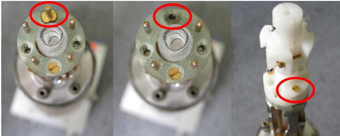
Figure 11.2: Mounting of a Solenoid Coil
