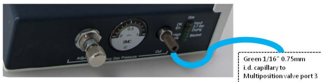
Figure 3.4: Connection Front Side
