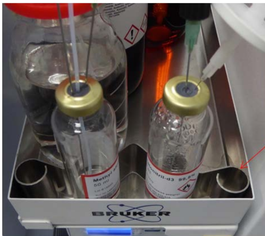
Figure 3.2: Metal Spring to Fix the Containers
