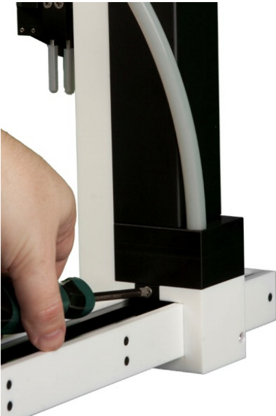
Figure 10.3: Attaching the Z-Drive to the Carriage.
