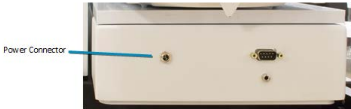
Figure 9.9: Power Connections for the Sample Stage
