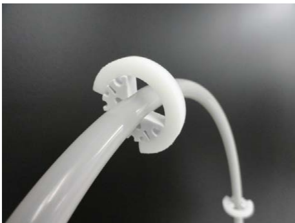
Figure 10.7: Tubing Tamer Properly Installed on Z-Drive Cable
