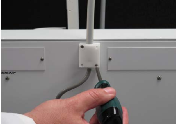
Figure 10.4: Attaching the Z-Drive Strain Relief Block
