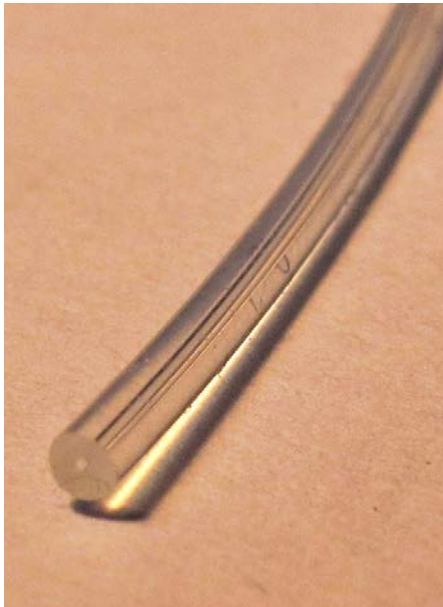
Figure 9.2: The tubing must be cut as near as possible to 90° ( extremely important )
