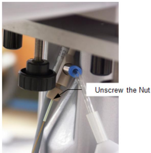
Figure 7.1: T-piece and Disconnected Outlet Capillary
