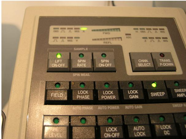
Figure 6.8: Activating the Sample Lift
