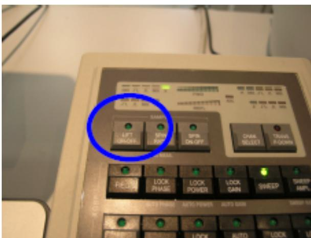
Figure 6.4: Switching Off the Sample Lift
