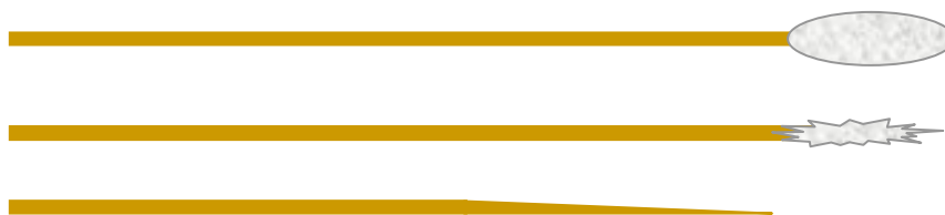
Figure 5. Cotton swabs on wood sticks are useful cleaning tools for MAS rotors and caps.
