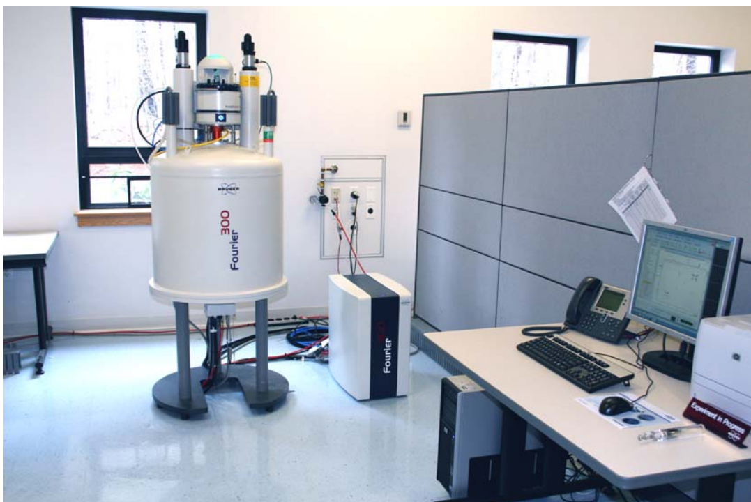
Figure 4.1: Room layout example of an installed Fourier system
