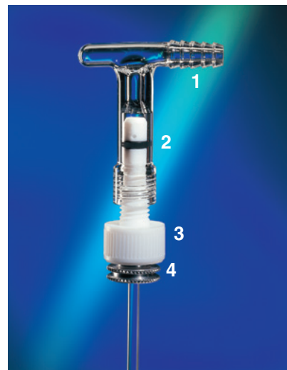
1: Glass Section; 2: Piston O-ring; 3: Piston Valve; 4: Aluminum Port Bushing
