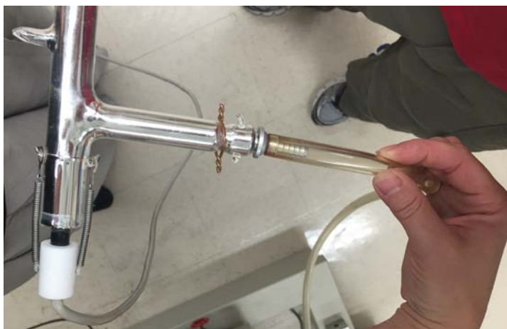
Figure 11. House Nitrogen gas line connected to vertical end of transfer arm
