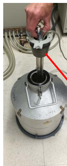
Figure 8. Dewar insert heater
