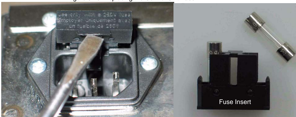
Figure 9.10. Replacing the Control Unit Fuse
