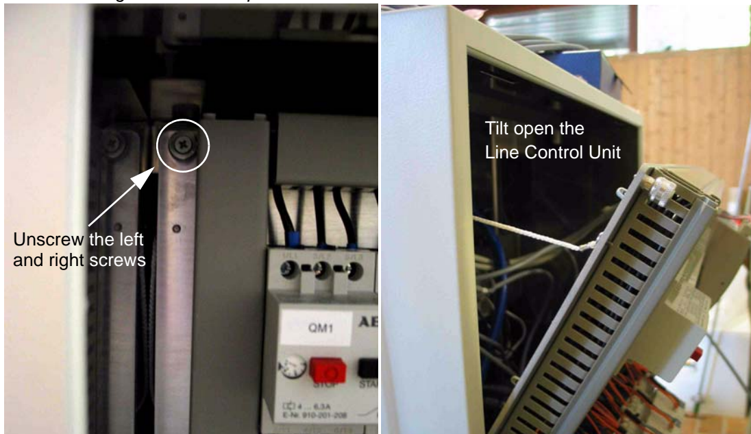
Figure 9.9. Tilt Open the Line Control Unit
