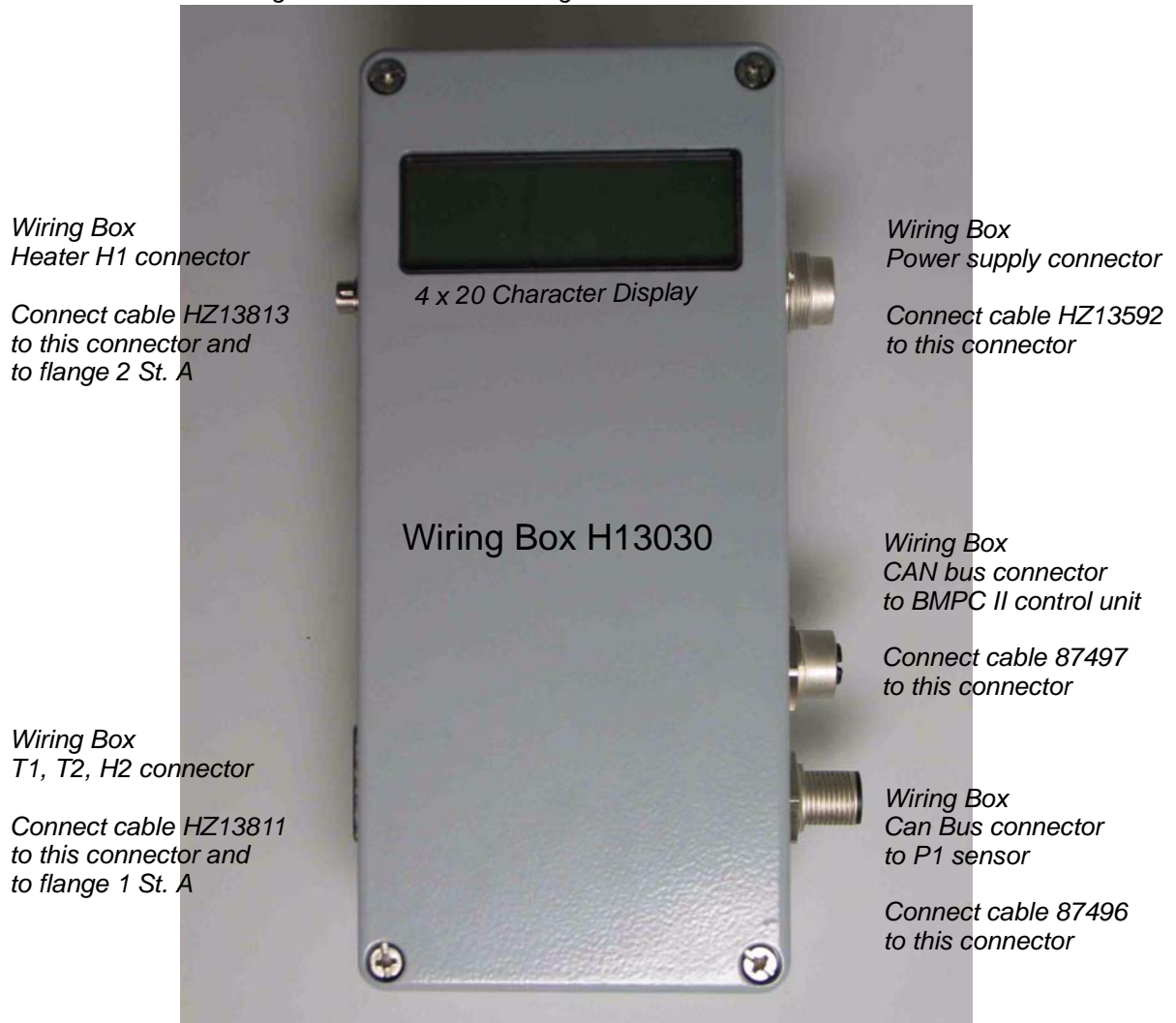
Figure 8.4. BMPC II Wiring Box
