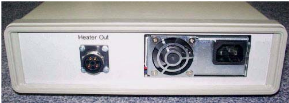
Figure 3.4. Rear View of the B-ACS Heater Supply 2
